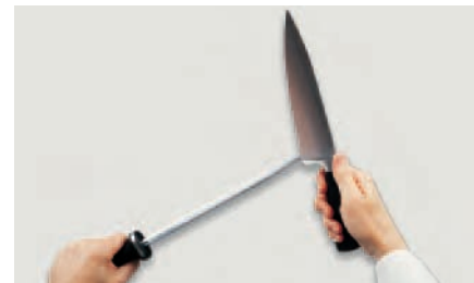
(a) Hold the steel and the knife away from your body. With the knife in a vertical position and at a 20-degree angle to the steel, touch the steel with the heel of the blade.
