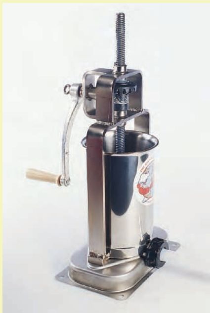
(a) A small sausage stuffer fitted with a medium nozzle. This stuffer holds 5 lb (2.3 kg) meat at a time.
