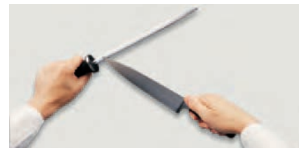
(c) Complete the movement. Do not strike the guard of the steel with the tip of the blade.
