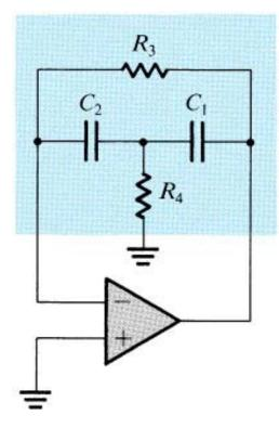
$$s^{2} + s\frac{\omega_{0}}{Q} + \omega_{0}^{2} = s^{2} + s\left(\frac{1}{C_{1}} + \frac{1}{C_{2}}\right)\frac{1}{R_{3}} + \frac{1}{C_{1}C_{2}R_{3}R_{4}}$$
