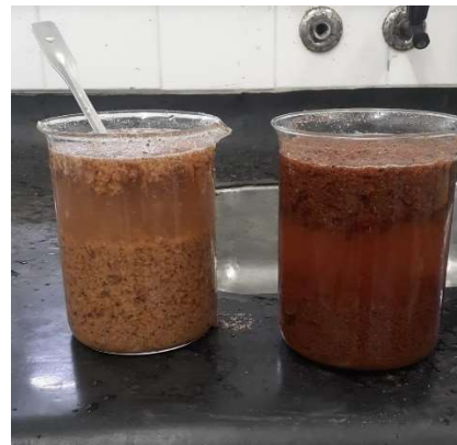
Figure 7. Whashing the samples with reagent water type IV.
