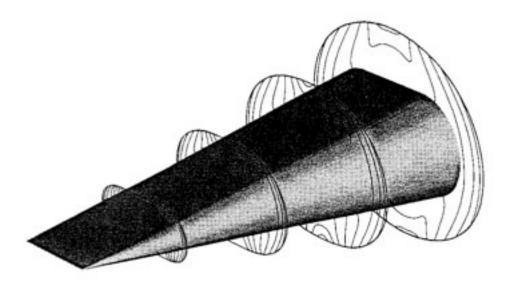
Figure 5. Wedge-cone pressure contours [7]
