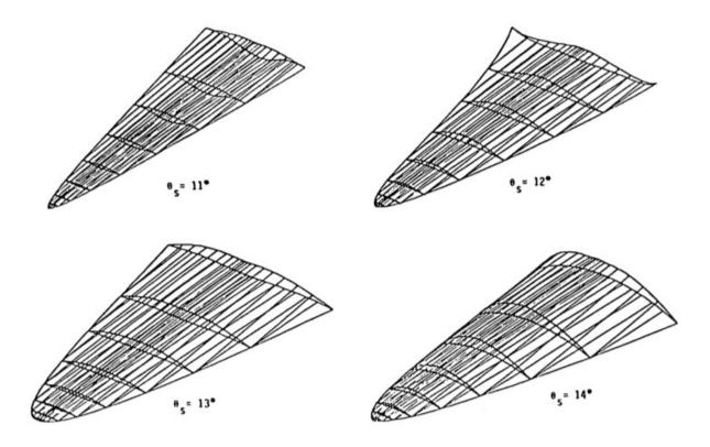
Figure 3. Hypersonic waveriders optimized for Mach 6 at varying shock cone angles [5]
