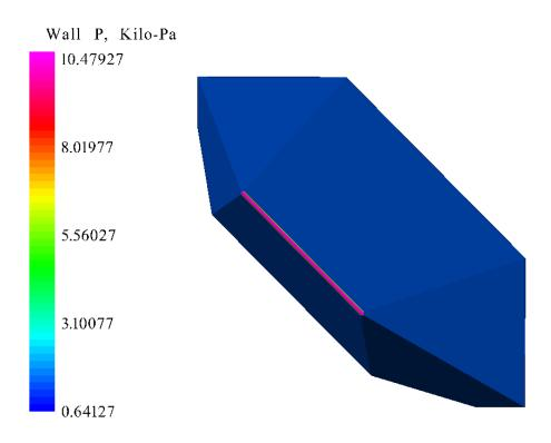
Figure 68. Proto-Waverider Pressure at Mach 5.73, 28.77 km Altitude, and 12° AOA
