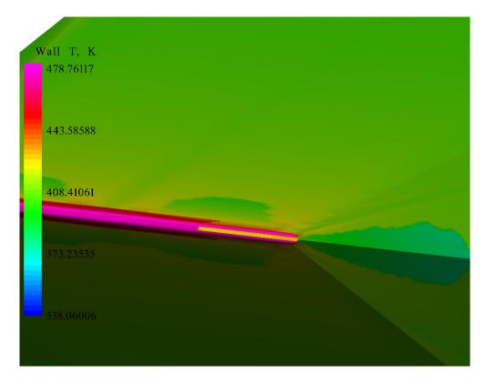
Figure 81. Proto-Waverider Nose Temp. at Mach 2.39, 28.24 km Altitude, and 0° AOA
