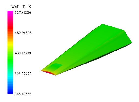
Figure 69. Proto-Waverider Temperature at Mach 2.59, 30.27 km Altitude, and 0° AOA
