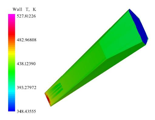
Figure 72. Proto-Waverider Bottom Temp. at Mach 2.59, 30.27 km Altitude, and 0° AOA
