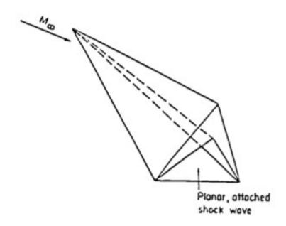
Figure 1. Simple caret wing waverider [4]
