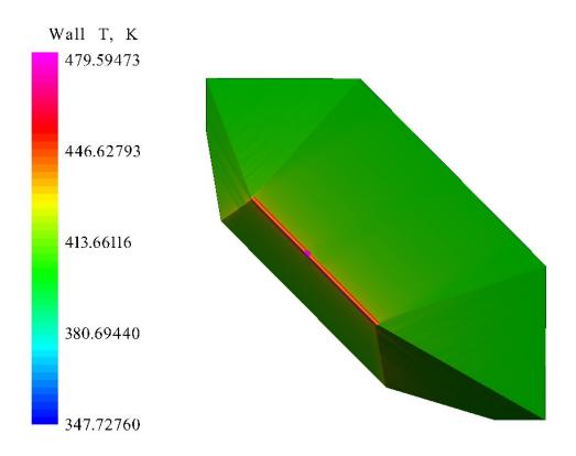
Figure 83. Proto-Waverider Temperature at Mach 2.39, 28.24 km Altitude, and 4° AOA
