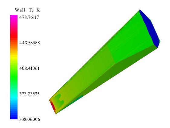
Figure 82. Proto-Waverider Bottom Temp. at Mach 2.39, 28.24 km Altitude, and 0° AOA
