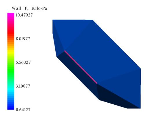
Figure 58. Proto-Waverider Pressure at Mach 6.85, 39.25 km Altitude, and 12° AOA
