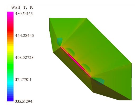
Figure 65. Proto-Waverider Temperature at Mach 5.73, 28.77 km Altitude, and 8° AOA
