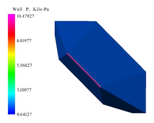
Figure 56. Proto-Waverider Pressure at Mach 6.85, 39.25 km Altitude, and 8° AOA
