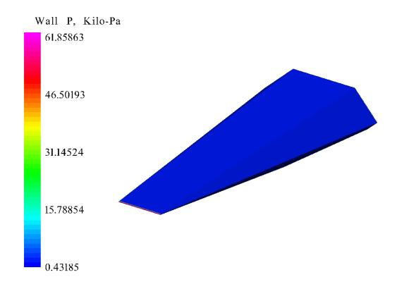
Figure 60. Proto-Waverider Pressure at Mach 5.73, 28.77 km Altitude, and 0° AOA
