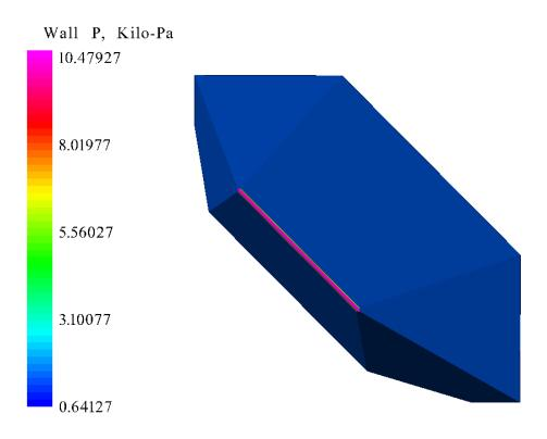
Figure 76. Proto-Waverider Pressure at Mach 2.59, 30.27 km Altitude, and 8° AOA
