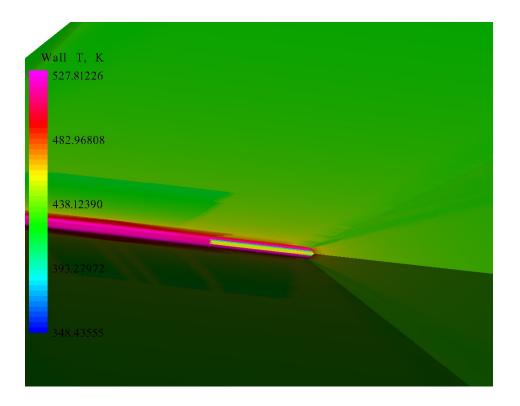
Figure 71. Proto-Waverider Nose Temp. at Mach 2.59, 30.27 km Altitude, and 0° AOA
