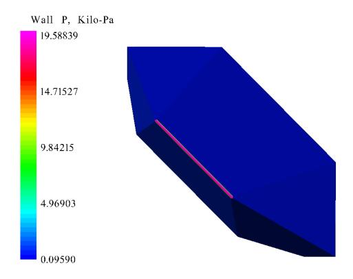
Figure 54. Proto-Waverider Pressure at Mach 6.85, 39.25 km Altitude, and 4° AOA
