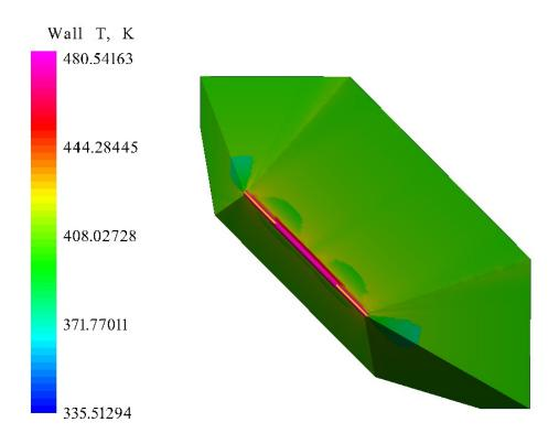
Figure 75. Proto-Waverider Temperature at Mach 2.59, 30.27 km Altitude, and 8° AOA
