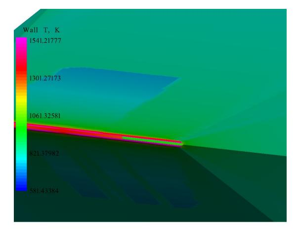
Figure 61. Proto-Waverider Nose Temp. at Mach 5.73, 28.77 km Altitude, and 0° AOA
