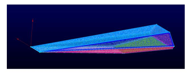
Figure 46. Diametric View of Waverider Mesh
