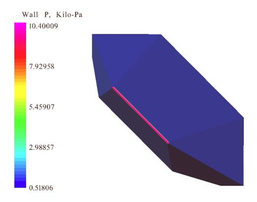
Figure 74. Proto-Waverider Pressure at Mach 2.59, 30.27 km Altitude, and 4° AOA
