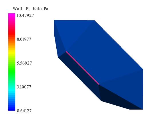
Figure 66. Proto-Waverider Pressure at Mach 5.73, 28.77 km Altitude, and 8° AOA
