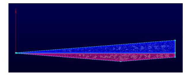
Figure 44. Side View of Waverider Mesh
