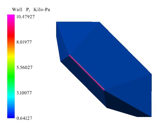
Figure 88. Proto-Waverider Pressure at Mach 2.39, 28.24 km Altitude, and 12° AOA
