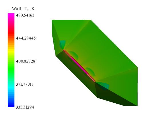
Figure 87. Proto-Waverider Temperature at Mach 2.39, 28.24 km Altitude, and 12° AOA
