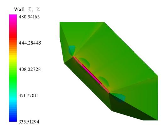
Figure 77. Proto-Waverider Temperature at Mach 2.59, 30.27 km Altitude, and 12° AOA
