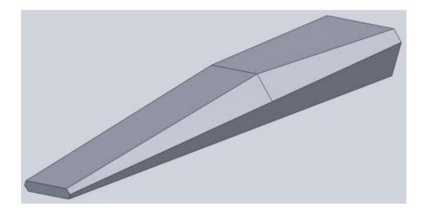
Figure 35. Isometric View of Proto-Waverider by Loft Method
