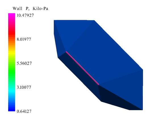
Figure 86. Proto-Waverider Pressure at Mach 2.39, 28.24 km Altitude, and 8° AOA
