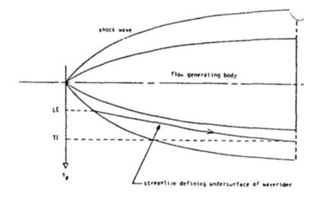
Figure 19. Leading Edge Cutting Streamline for Waverider Body [15]
