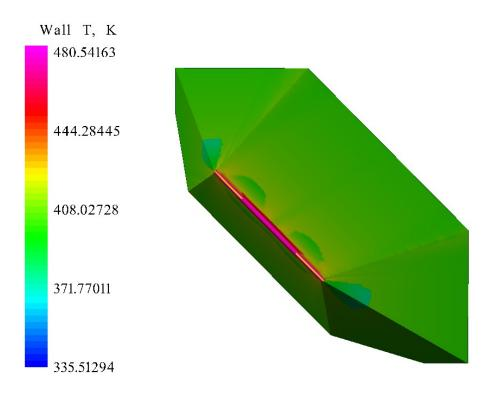
Figure 67. Proto-Waverider Temperature at Mach 5.73, 28.77 km Altitude, and 12° AOA
