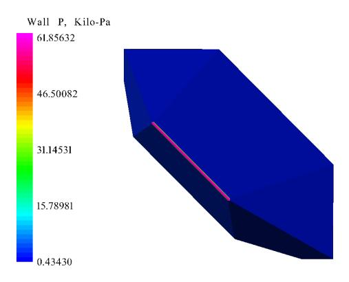
Figure 64. Proto-Waverider Pressure at Mach 5.73, 28.77 km Altitude, and 4° AOA
