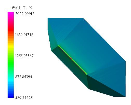
Figure 53. Proto-Waverider Temperature at Mach 6.85, 39.25 km Altitude, and 4° AOA
