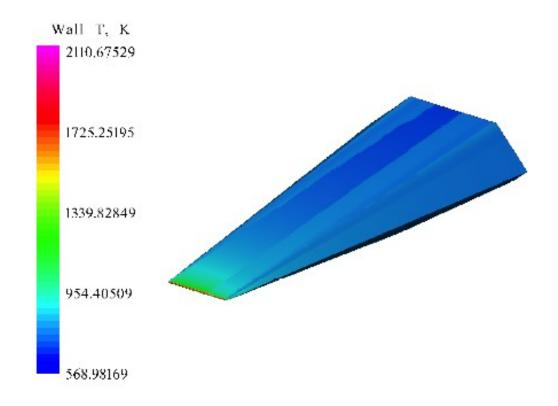
Figure 49. Proto-Waverider Temperature at Mach 6.85, 39.25 km Altitude, and 0° AOA
