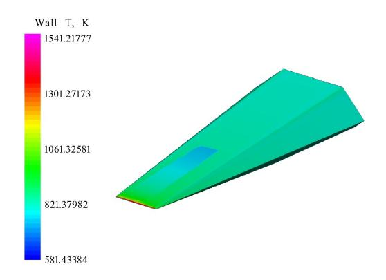
Figure 59. Proto-Waverider Temperature at Mach 5.73, 28.77 km Altitude, and 0° AOA
