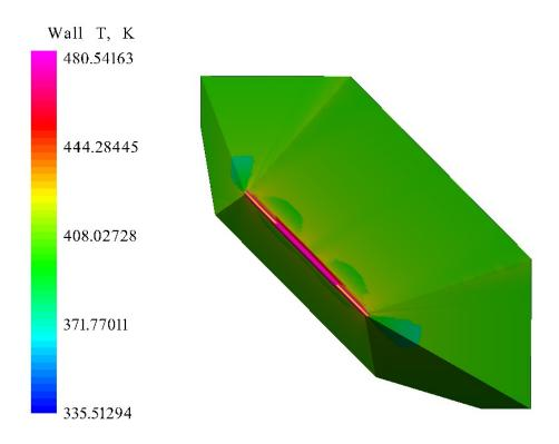
Figure 55. Proto-Waverider Temperature at Mach 6.85, 39.25 km Altitude, and 8° AOA
