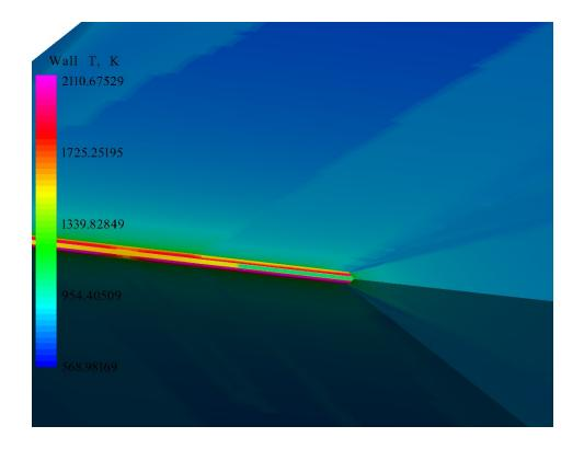
Figure 51. Proto-Waverider Nose Temp. at Mach 6.85, 39.25 km Altitude, and 0° AOA
