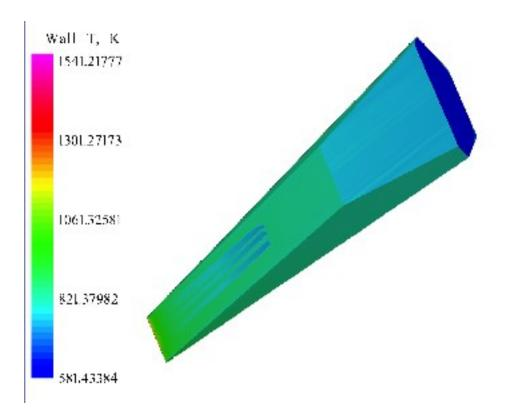
Figure 62. Proto-Waverider Bottom Temp. at Mach 5.73, 28.77 km Altitude, and 0° AOA
