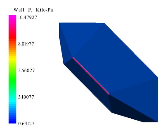
Figure 78. Proto-Waverider Pressure at Mach 2.59, 30.27 km Altitude, and 12° AOA
