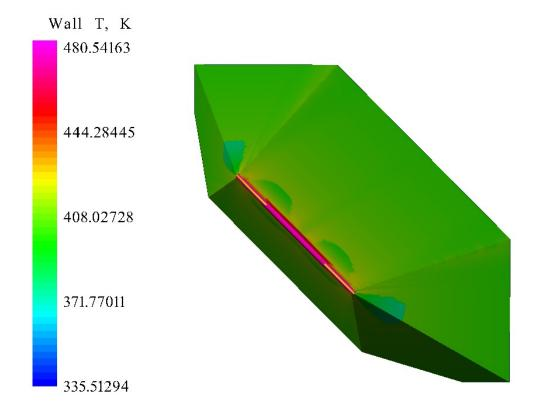
Figure 85. Proto-Waverider Temperature at Mach 2.39, 28.24 km Altitude, and 8° AOA
