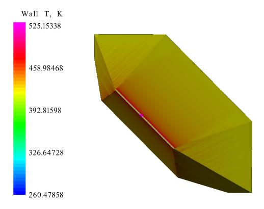
Figure 73. Proto-Waverider Temperature at Mach 2.59, 30.27 km Altitude, and 4° AOA
