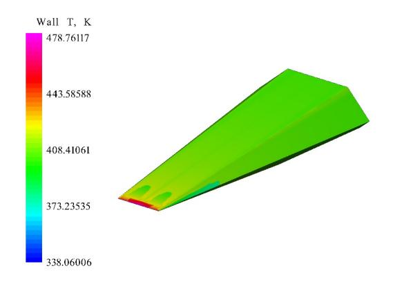
Figure 79. Proto-Waverider Temperature at Mach 2.39, 28.24 km Altitude, and 0° AOA
