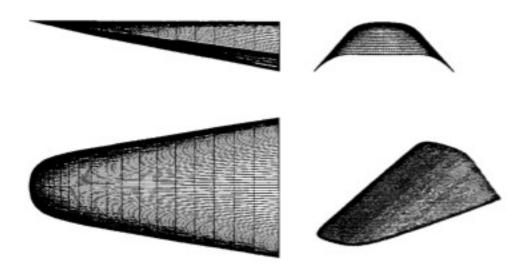
Figure 4. Wedge-cone hypersonic waverider [7]
