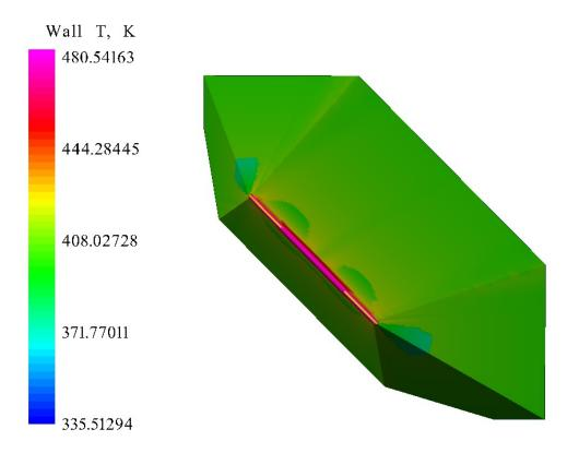
Figure 57. Proto-Waverider Temperature at Mach 6.85, 39.25 km Altitude, and 12° AOA
