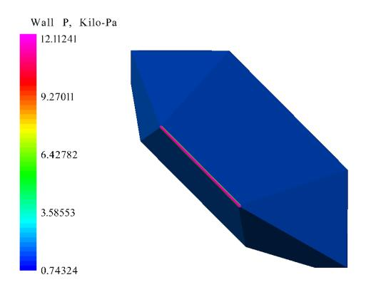
Figure 84. Proto-Waverider Pressure at Mach 2.39, 28.24 km Altitude, and 4° AOA
