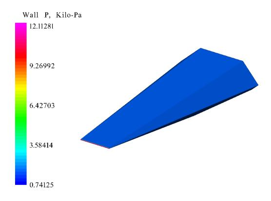
Figure 80. Proto-Waverider Pressure at Mach 2.39, 28.24 km Altitude, and 0° AOA
