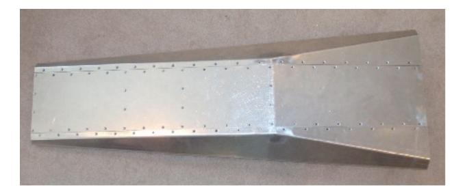
Figure 23. Bottom View of Proto-Waverider
