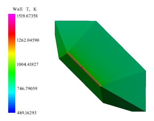
Figure 63. Proto-Waverider Temperature at Mach 5.73, 28.77 km Altitude, and 4° AOA
