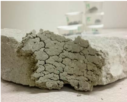
Figure 2-8. The texture of the bentonite in Test 8 which had swelled into the inner slot.
