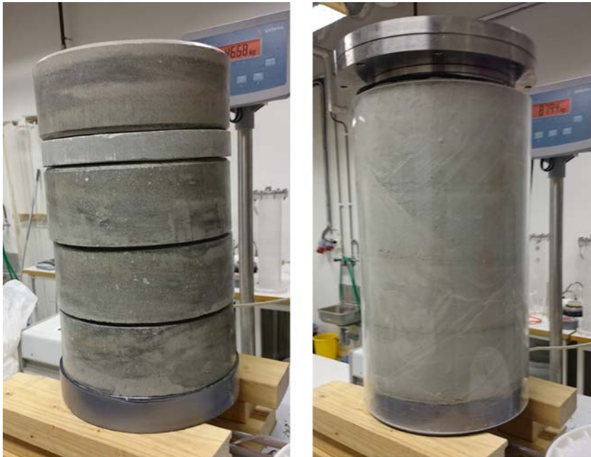
Figure 2-2. Left: Four bentonite rings and a massive block stacked on top of each other. Right: The full set-up before starting the experiment.
