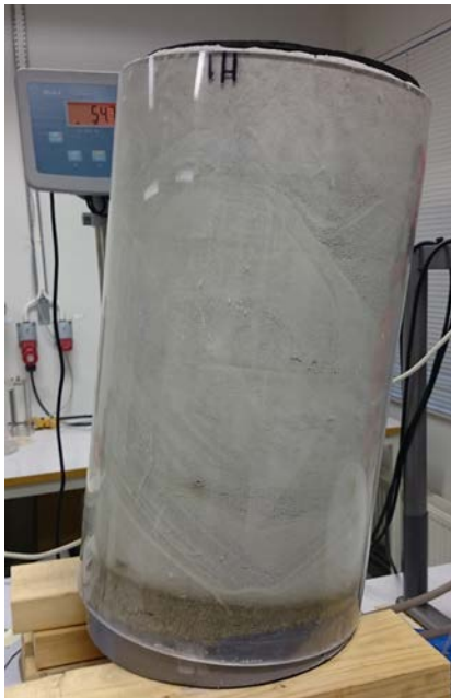
Figure 2-4. Massive swelling occurred during the course of test. Moreover, the swelling was uneven, causing tilting of the set-up.
