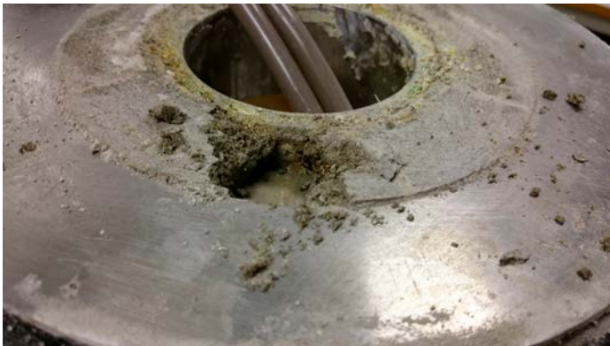
Figure 2-19. Sampling of the bentonite in the ring through which water was fed in Test 9.
