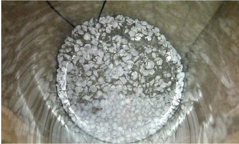
Figure 3-2. State of the pellets filling in test Room2 in Birgersson and Goudarzi (2013). The photo shows the pellets filling from above; the water source is below, and the direction of the vapor transport is out of the picture. A clear division is seen between very wet pellets (the top part) and dry pellets (bottom). The water uptake occurred in such a way that the wet part “propagated” across the filling until eventually all pellets were wet. During the course of this process, a substantial amount of vapor was able to pass through the dry part of the pellets filling without being taken up by the dry bentonite.
