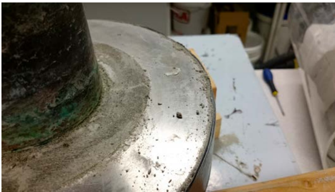
Figure 2-18. Top of bentonite ring through which water was fed in Test 9.
