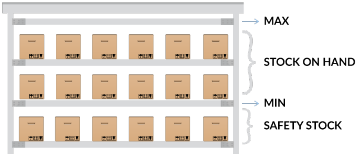
Figure 21. Min/Max inventory replenishment system. Developed by LINCS in Supply Chain Management Consortium.
