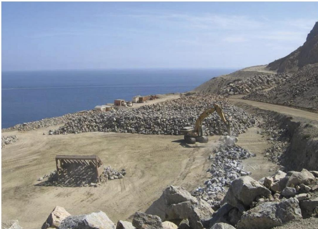
Rock production at Pebbly Beach Quarry. Large rocks were broken into smaller rocks by the Breaker (right) and small rocks were separated out by the Grizzly (left).
