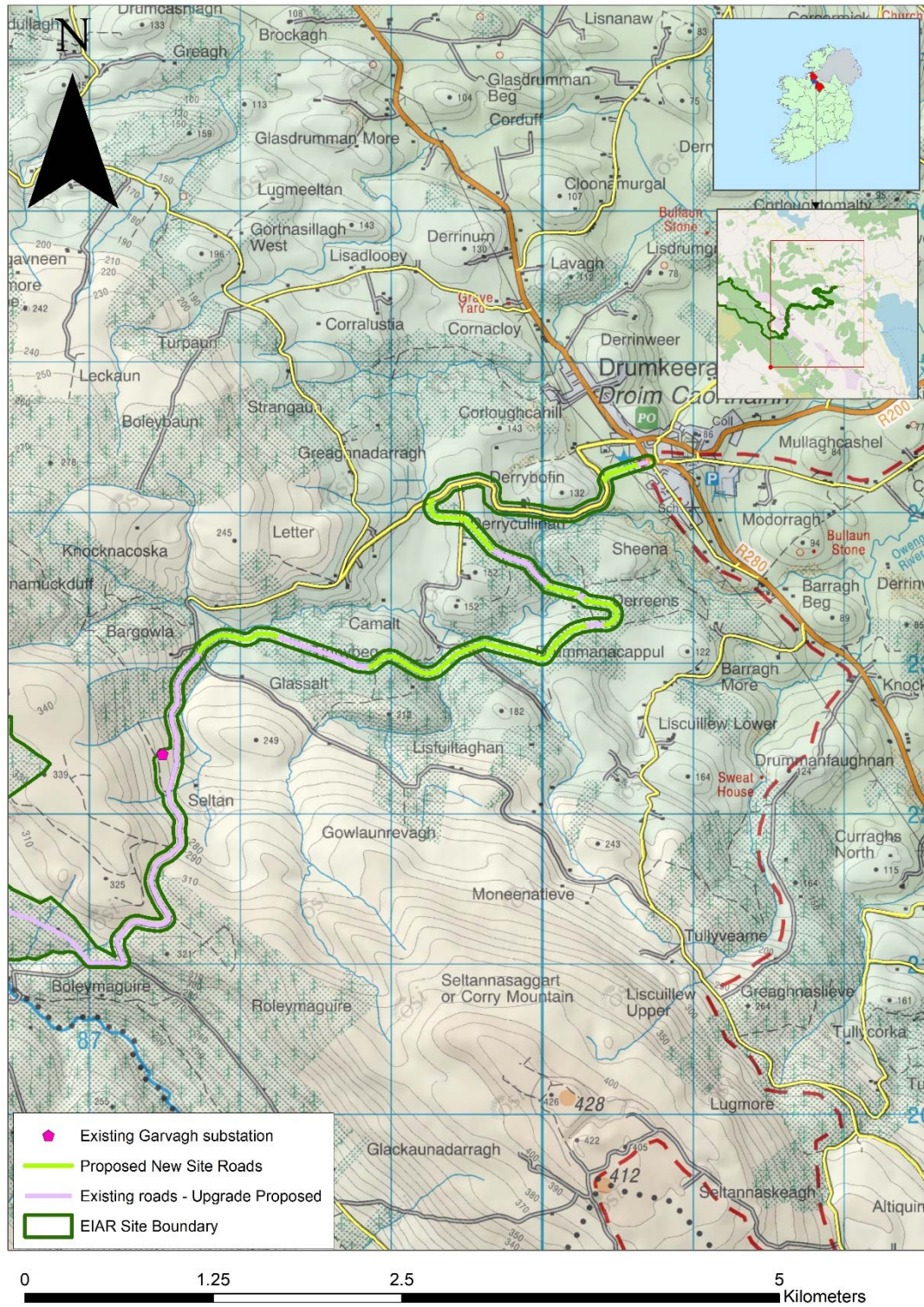
Figure 13-22 Proposed construction access road between R280 Regional road and proposed core wind farm site.
