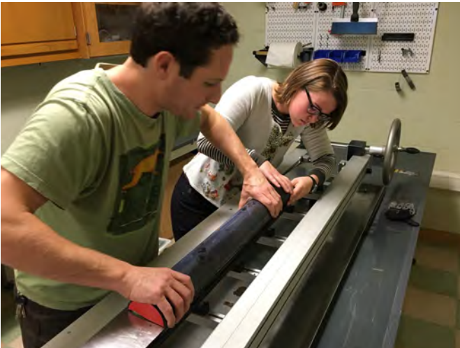
Emma Harnisch 18 splitting her Cooks Pond core for analysis on the ITRAX scanner at UMASS with help from Brian Yellen (UMASS).
