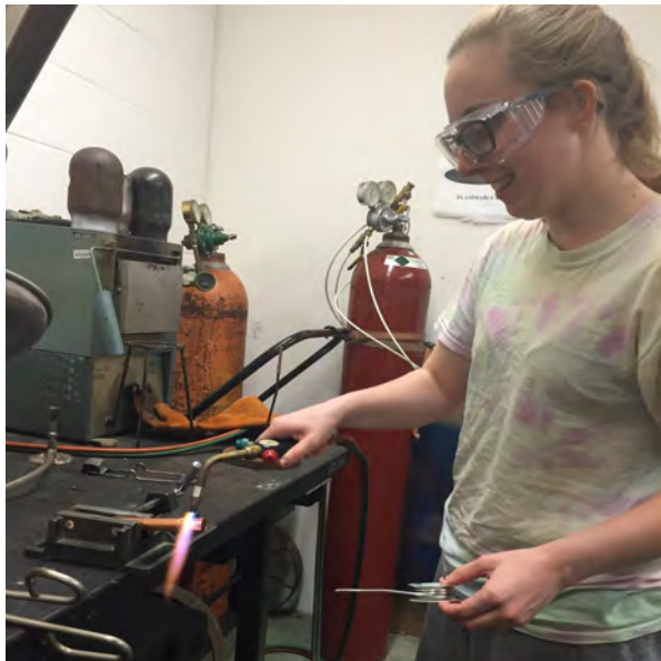
Sarah Dickson ('16) solders an end cap to a copper pipe with lead-based solder in preparation of lead-leaching experiments for Aqueous Geochemistry.
