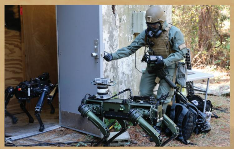
A service member participates in a simulated CBRN training scenario during RDAX Dragon Spear 2023. The service member wears the uniform integrated protection ensemble family of systems general purpose (UIPE FOS GP) suit and M50 joint service general purpose mask (JSGPM) and uses robot dogs equipped with CBRN sensors. Photo by Alex Hillman.
