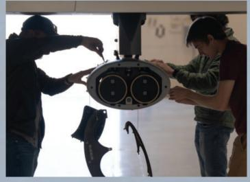
Altius employees perform pre-flight checks on a dual launch pod attached to an MQ-9 Reaper before an Airborne Adaptive Enterprise (A2E) demonstration at Cannon Air Force Base, N.M., Nov. 28, 2023. Adaptive Airborne Enterprise will utilize large and small uncrewed aircraft systems at scale, including a mix of attritable and expendable systems with modular payloads. Photo by U.S. Air Force Staff Sgt. Nicholas Swift.
