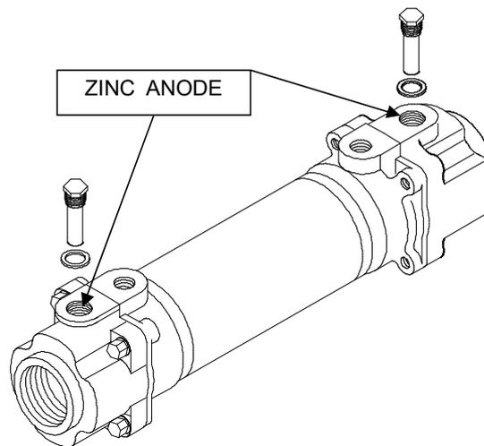
The oil Cooler is fixed above the case cover with bolts, and cools the oil supplied from the hydraulic pump before leading it into the secondary oil filter. Oil Cooler contains the alloy (of aluminium and brass) pipe which is strong against corrosion. In addition, zinc anodes are put into the oil cooler.
