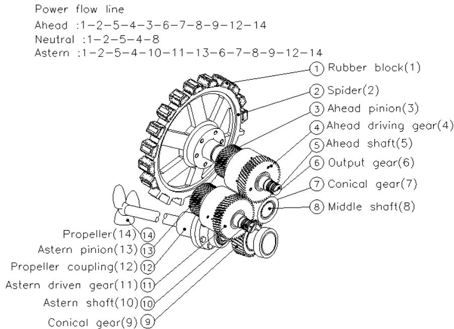
[Fig-2] Marine Transmission Power Flow
