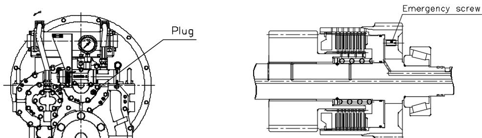
[Fig-7] Position of Emergency Screw
