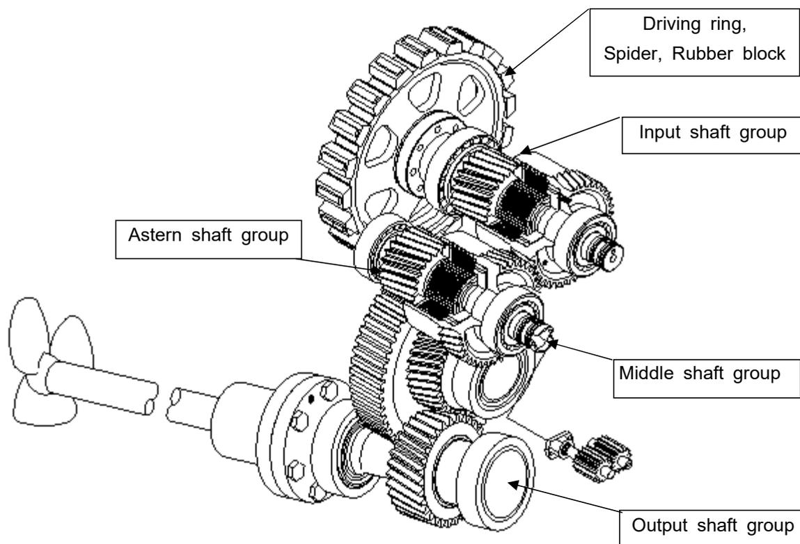
[Fig-1] Marine Transmission Construction
