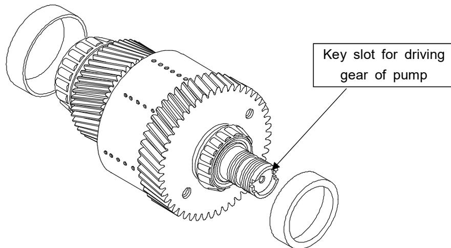
The astern shaft assembly has the same parts as those which the input shaft assembly has, except that the former has no spline in the front and has the hydraulic pump driving device in the rear end.
