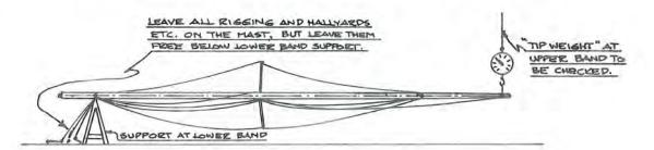
IF "TIP WEIGHT" IS FOUND TO BE LOWER THAN 11 KG, EITHER MAST WEIGHT OR CENTRE OF GRANTY IS IN THE DANGER ZONE", AND IT WOULD BE ADVISABLE TO STRIP MAST FOR FUETHER CONTROL
