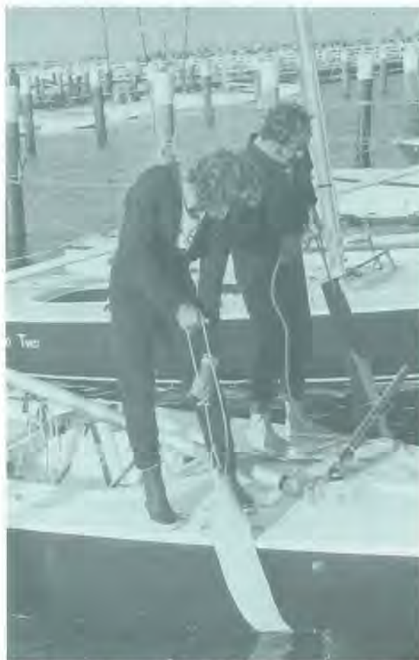
The Brazilian Schmidt Brothers scrubbing the bottom of "Osprey" at Kiel 1972. This is a workable way to do it when not allowed to haul out during an event.
