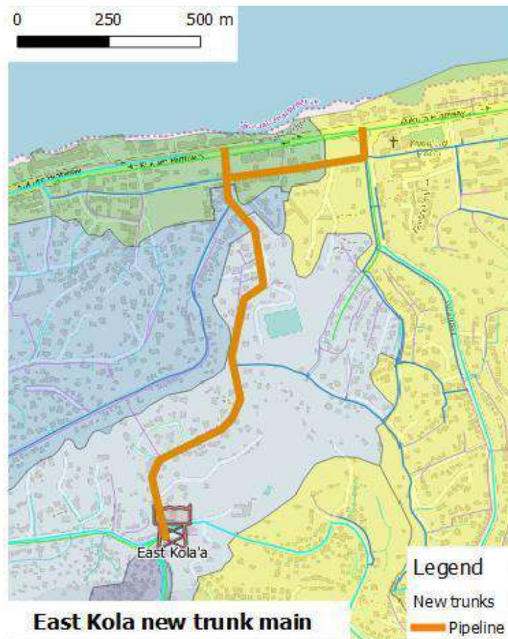
Figure 3-4: Proposed Location of East Kola'a Trunk Main (on landscape page by itself)
