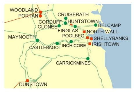
Figure 8-2: Dublin Area 220 kV Transmission System
