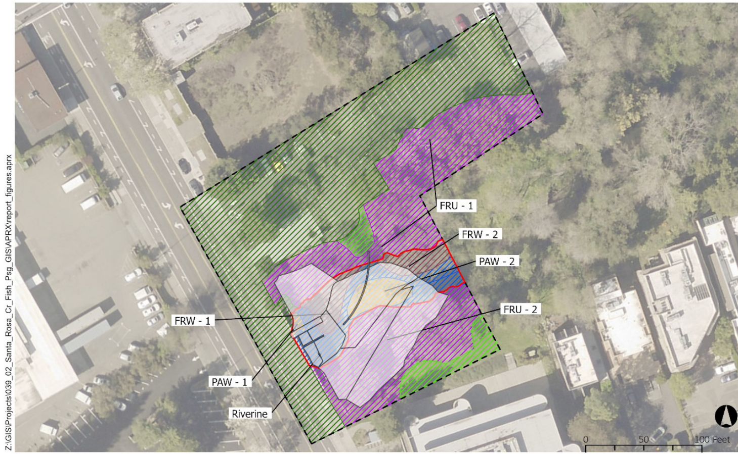
Figure 3.4-3. Proposed Project Features Permanent Impacts at E Street Bridge Fishway Extension Site.
