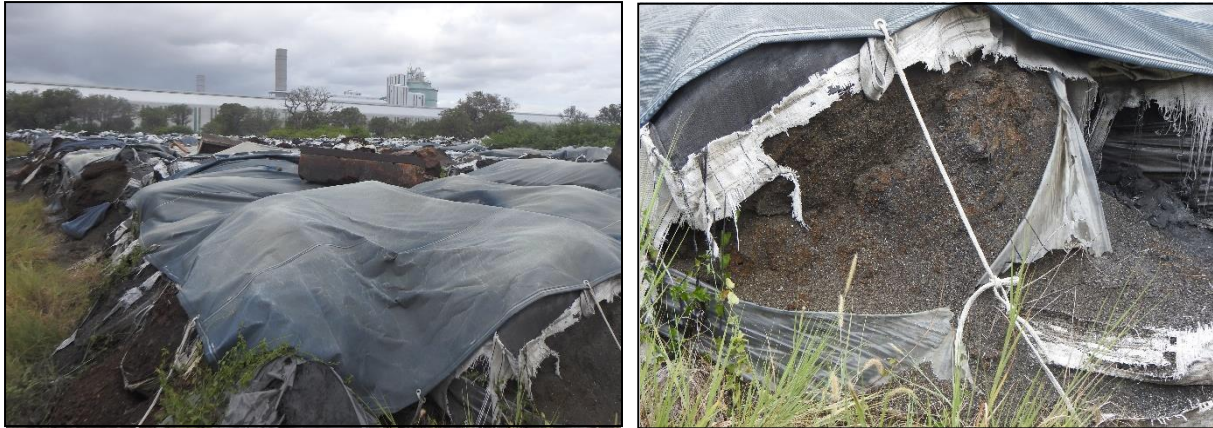
Figure 4-1 Basement and carbonaceous material stockpiled on the Mozal smelter site
