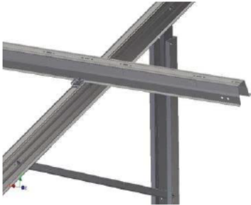
Mount purlin perpendicular to girder
