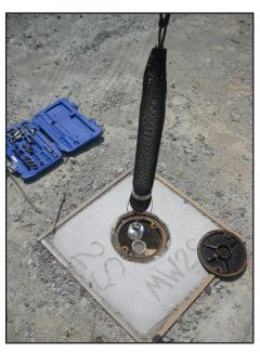
The passive diffusion bag technique is used on environmental restoration sites at Fort Bragg, North Carolina, as a less invasive option for sampling groundwater. Once the bag is deployed, it is removed and tested for volatile organic compounds. (U.S. Army photo)
