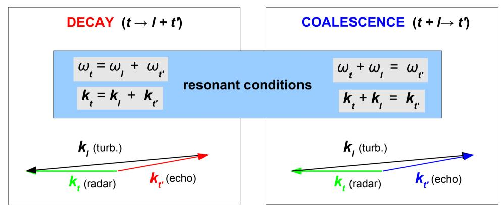
• radar wave  $\boldsymbol{\omega}_{t}$  is scattered into two satellites:
