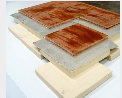
Floor deck system used at Weston Super-Mare Pier
