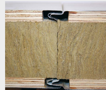
Plywood lined non combustible panel
