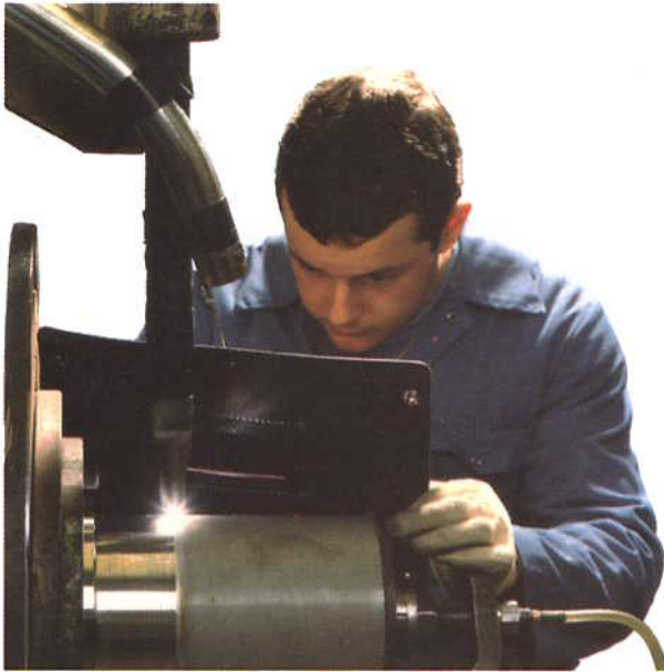
Fig. 22-8 Tungsten inert gas welding.
