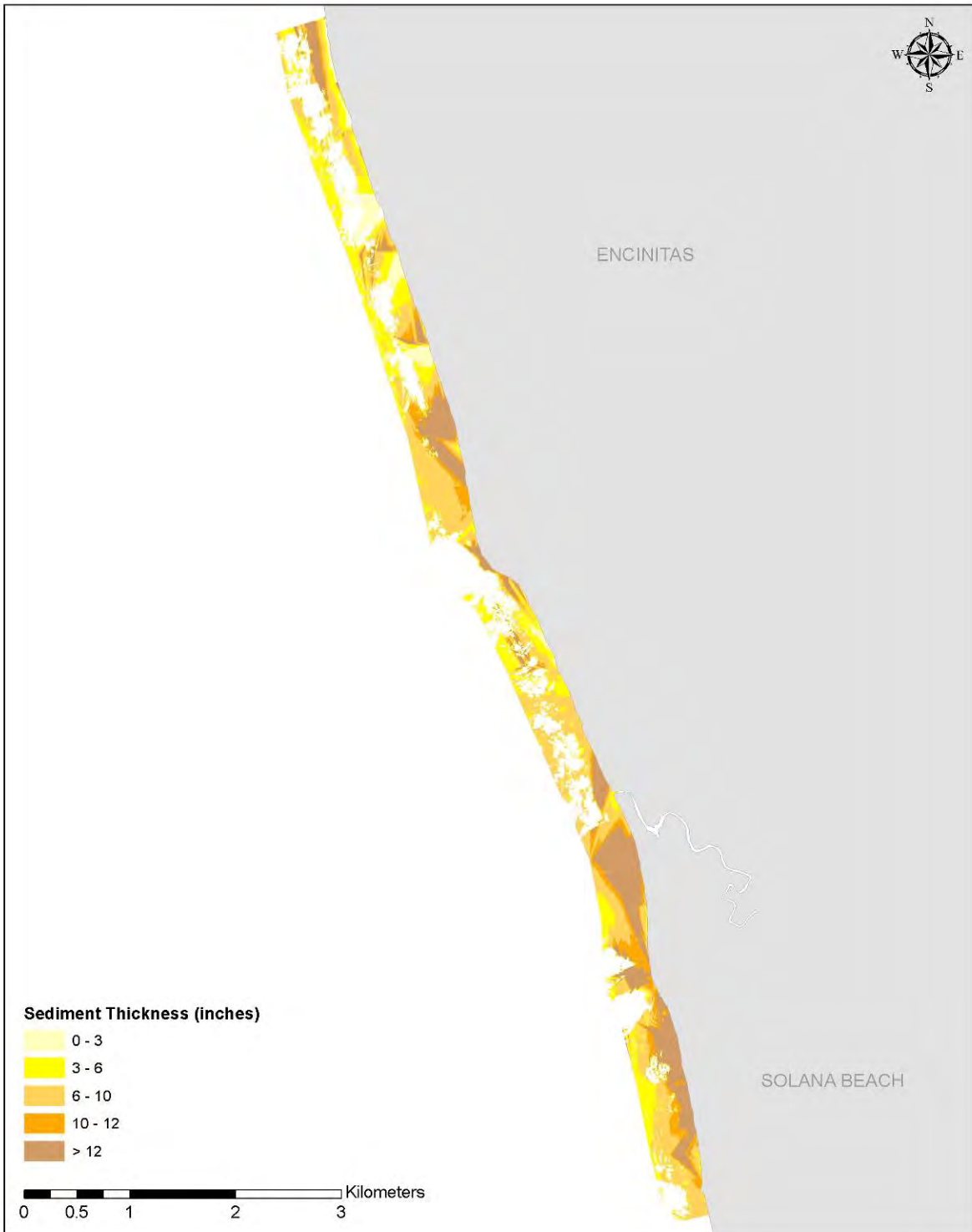
Figure 4.4-8 “Natural Variation” sediment thickness based empirical coastal profile data collected from 1996 to 2008.
