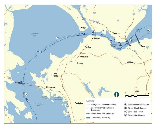
Figure 2-11. Buried/Underwater Cables.
