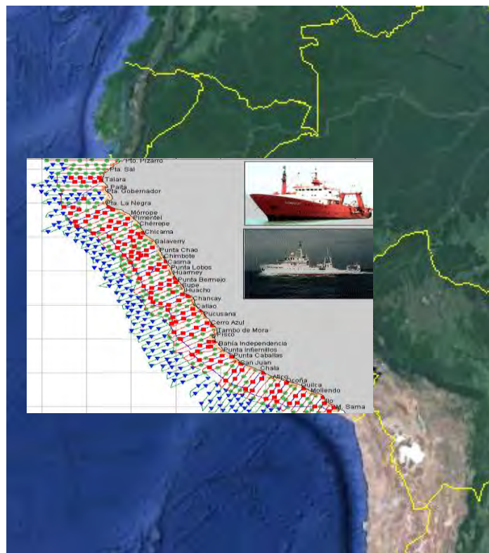
Figure 4. Example of a standard survey in Peru. Transects are separated by 15 NM; fishing samples are collected either regularly (to get biological samples in every region) or each time particularly interesting detections are observed; CTD and plankton stations are performed at predefined points. In this example, the survey was performed simultaneously by two vessels: R/ V Olaya (transects in red) for the inshore area and R/V Humboldt (transects in blue) for the offshore area. Fishing samples are performed by these two vessels plus fishing boats hired for the duration of the survey to sample the coastal area out of range of the two R/V.
