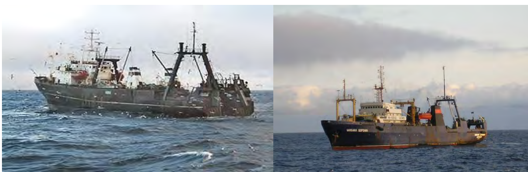
Figure 2. Examples of pelagic trawlers from the USSR. Note that these two particular trawlers BATM, RTMK-S of 5700 and 9260 t displacement respectively, were also used for exploration and research surveys in the 70s. From Nesterov, 2006
