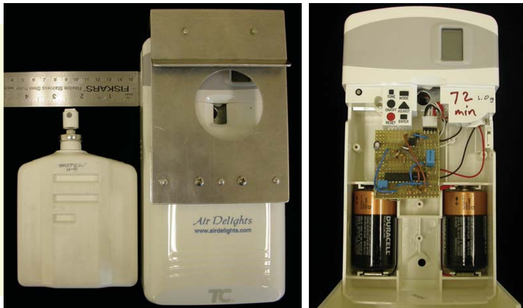
Figure 26.4 —Puffer devices adapted for use with bark beetle semiochemicals from Air Delights (Air Delights, Inc., Beaverton, Oregon) lavatory air fresheners. Adaptations include a timer to vary the period between puffs, thereby determining the daily rate of semiochemical released from the reservoir. (Adaptations made by USDA Forest Service personnel at the Missoula Technology Development Center, Missoula, Montana). (photograph by B. Strom)
