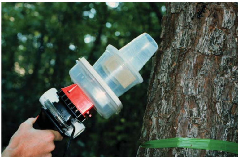
Figure 28.7 —Dustbuster® cordless vacuum, modified for parasitoid collection
