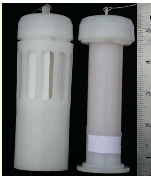
Figure 26.5 —Prototype active, point-source releasers (pumps) developed by Med-e-Cell, Inc. (San Diego, California) to release bark beetle semiochemicals. Southern pine beetle verbenone releaser (left) was designed to release about 300 mg per day for 45 days. Western bark beetle version (right) was designed to release about 100 mg of verbenone per day for 3-4 months. Testing of performance in field applications has not been completed. (photograph by B. Strom)
