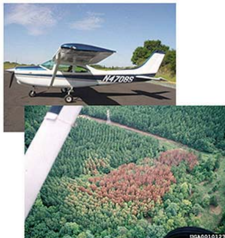
Figure 18.1— Sketchmapping forest pest infestations. Sketchmapping is a remote sensing technique of observing forest change events from an aircraft and documenting them manually on a map. (images by McConnell and others 2000, lower left photograph by Andrew J. Boone, www.forestryimages.org)
