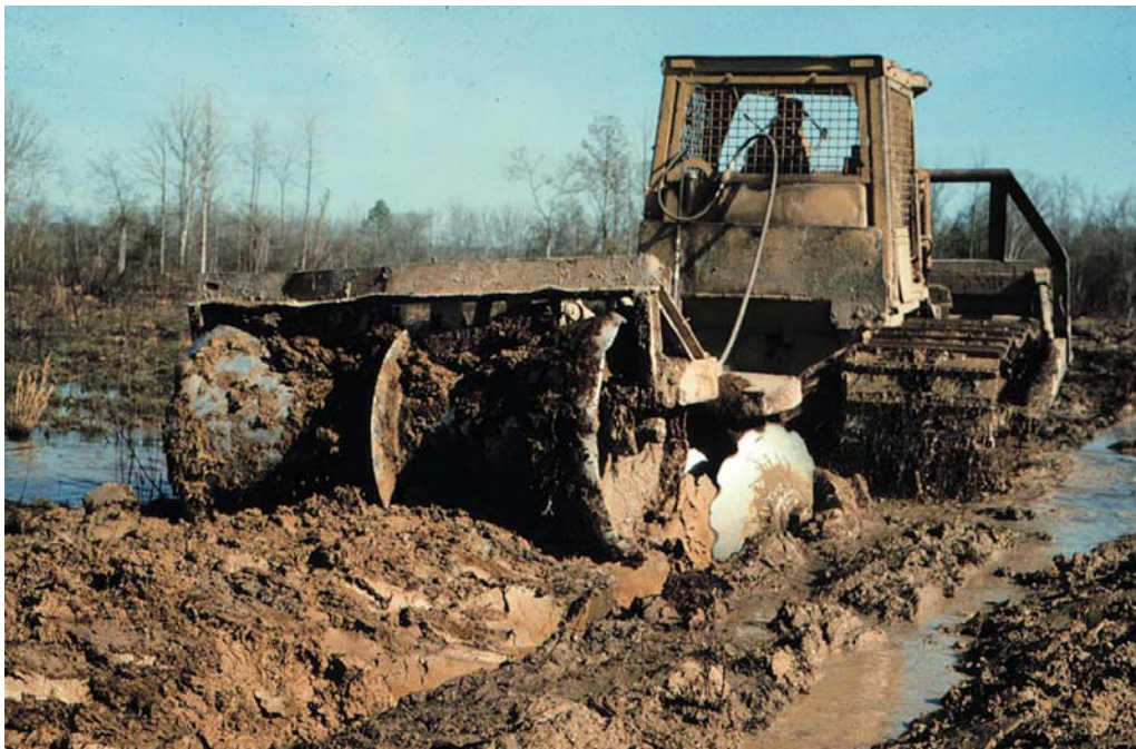
Figure 23.10 —Bedding as a final step in site preparation prior to planting on an upper west Gulf Coastal Plain site in Bradley County, Arkansas. (USDA Forest Service photograph by James M. Guldin)
