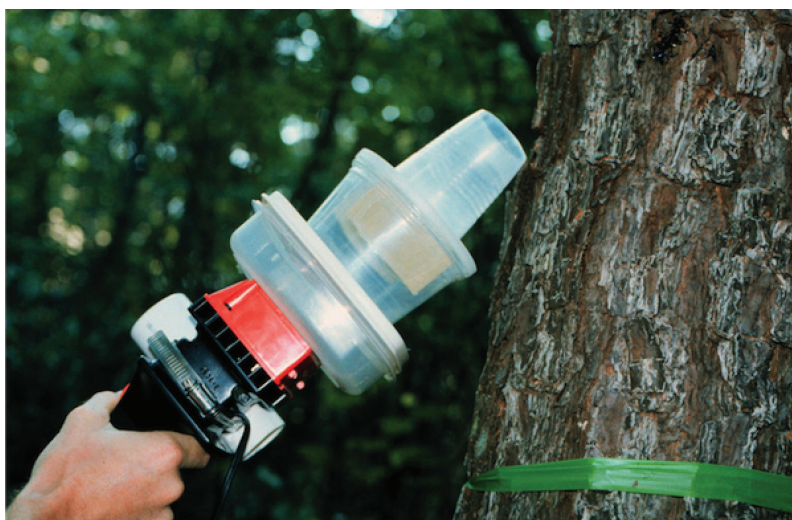
Figure 28.7 —Dustbuster® cordless vacuum, modified for parasitoid collection
