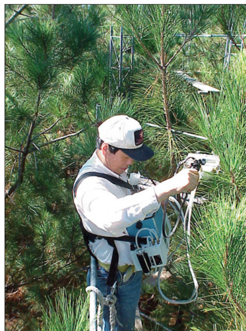
Tower system on the Palustris Experimental Forest provides access to the crowns of loblolly pines to evaluate physiology in response to stand management treatments in support of climate change initiatives.
