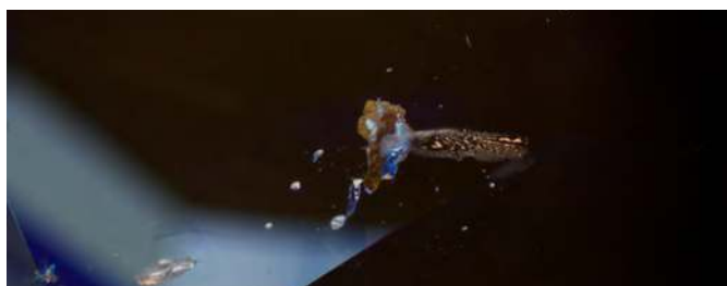
△ Figure 2: Surface-reaching rutile inclusion on which age-dating analysis was successfully carried out. Photo: M.S. Krzemnicki, SSEF
