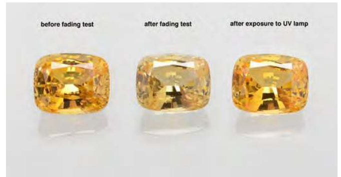
△ Figure 2: Yellow sapphire of >50 ct with unstable (reversible colour), seen before fading test (left), after fading test (middle), and after exposure to UV radiation (right). Photos: J. Kaysongkham, SSEF
