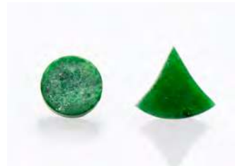
△ Figure 3: Two of a series of jadeite-looking stones sent for testing to SSEF. The round polished slab (left) is dominantly consisting of jadeite, whereas chemical and Raman microspectroscopic analyses revealed that the triangular specimen is dominated by omphacite, thus identified as omphacite-jade on our report.
