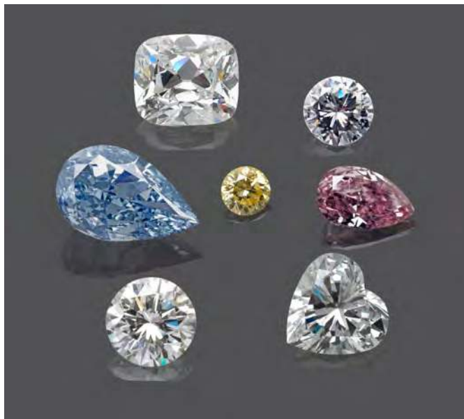
△ Figure 1: Seven colourless and fancy-colour diamonds (up to 3.03 ct) of various natural or synthetic origins are shown here. The top-right and bottom-left round brilliants are HPHT- and CVD-grown, respectively, and the other diamonds are natural. The confident separation of both natural and synthetic diamonds is critical to maintaining consumer confidence in the trade. Composite photo by Luc Phan, SSEF.
