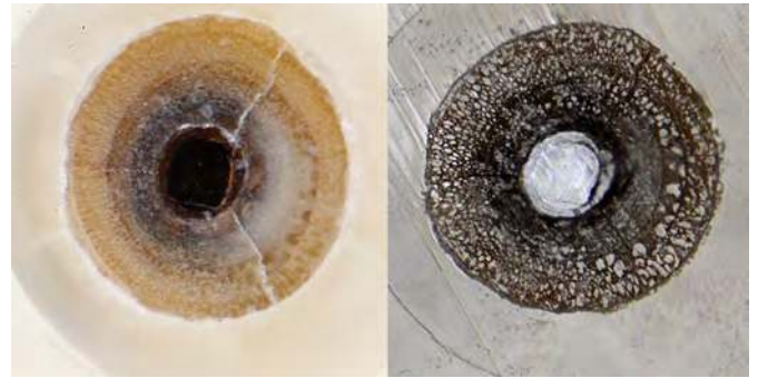
△ Figure 2: Microphotos of the core section in normal light and reflected light, revealing the black cube Fe-oxide grain in the centre, surrounded by a thin layer of dark brown Fe-hydroxide and radially arranged calcite columns with brownish organic matter. Photos: M.S. Krzemnicki, SSEF
