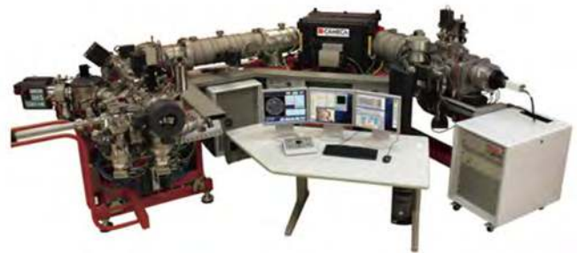
△ Figure 2: SwissSIMS Cameca IMS 1280-HR at the University of Lausanne. Photo: UNIL
