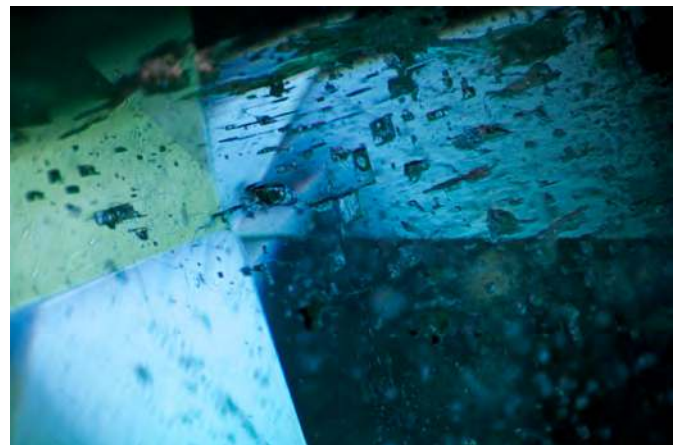
△ Figure 2: rectangular to comma-shaped fluid inclusions in an emerald from Ethiopia. The different colours in this photo are an effect of the pleochroism of emeralds. Photo: M.S. Krzemnicki, SSEF
