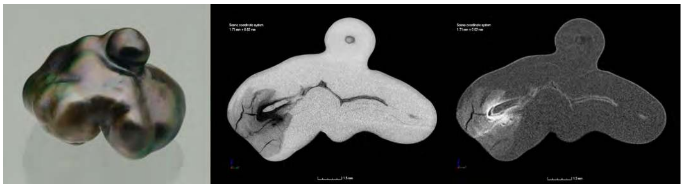
△ Figure 2: Non-beaded cultured pearl from Pinctada margaritifera (so-called 'Keshi cultured pearl') with a comparison of a section visualised by X-ray tomography (left) and neutron tomography (right). Photos: C. Hanser
