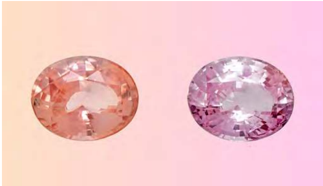
△ Figure 1: Fancy sapphire recently found in Madagascar showing an unstable colour, shifting from pinkish orange (padparadscha-like) to pink after a fading test. Photo: SSEF
