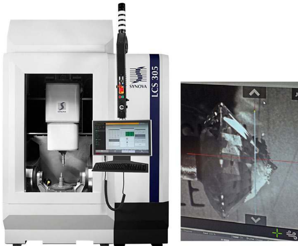
△ Figure 4: The SYNNOVA LCS 305 sawing device (left image) is a 5 axes water-guided laser-MicroJet machine which enables very precise ( \pm 0.1^\circ ) cutting profile. The precise positioning of the stone (right image) is observed via the help of a digital camera. Please note the white substance lying at the culet side of the stone enables the laser to easily penetrate into the stone. Photo: Synova.
