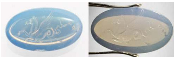
△ Figure 4: A comparison of the Roman sapphire intaglio in reflected light (left) and transmitted light (right) reveals the different colour appearances of the sapphire (bluish grey and greyish brown, respectively). Photos by M. S. Krzemnicki, SSEF.
