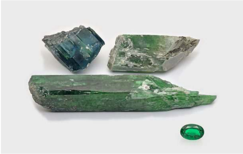
△ Figure 1: Spodumene crystals (longest item about 50 cm long and 5.9 kg heavy) submitted to SSEF as new 'emeralds' from Pakistan shown here together with a faceted emerald from Pakistan (magnified size). Photo: L. Phan, SSEF.
