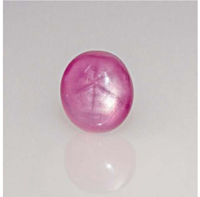
△ Figure 1: Trapiche-like pattern of pink sapphire (8.55 ct) treated with lead (Pb) glass. Photo: V. Lanzafame SSEF.
