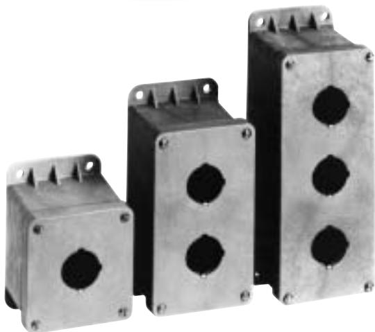
Wall mount pushbutton enclosures are molded from gray, engineered thermoplastic material that is resistant to most corrosive agents. Universal pushbutton holes are designed to accommodate all standard oil-tight pushbuttons, switches and pilot lights. A grounding plate is included on the cover. Auxiliary devices must be rated for appropriate NEMA applications.
