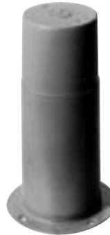
HOLFORM nonmetallic concrete sleeve forms are the easy way to form holes in concrete. They install in seconds with nails, screws or staples and are easily removed. Concrete will not adhere to them. HOLFORMS are adjustable to any slab thickness.
