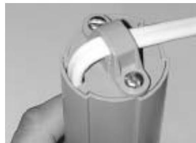
**5.** Secure wire clamp on bottom of tube.
