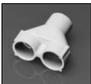
The 3/4" Y Fitting provides for in and out service from a single 1" port, and allows for two 3/4" parallel conduit runs to adapt into a single conduit body port.
