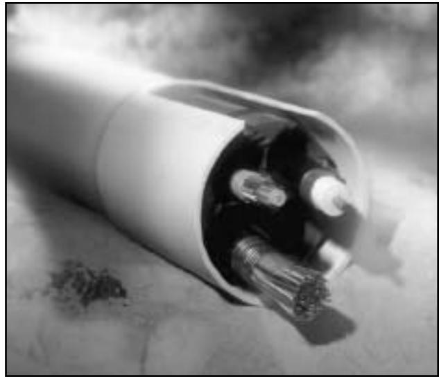
A 1/4" composite rope (braided polyethylene over braided polyester) was blown into the innerduct of Carlton's Multi-Gard. The force required to pull the rope through the 4,900 feet was 27 pounds. This force was measured after the rope rested in the flooded innerduct for more than 10 hours.
