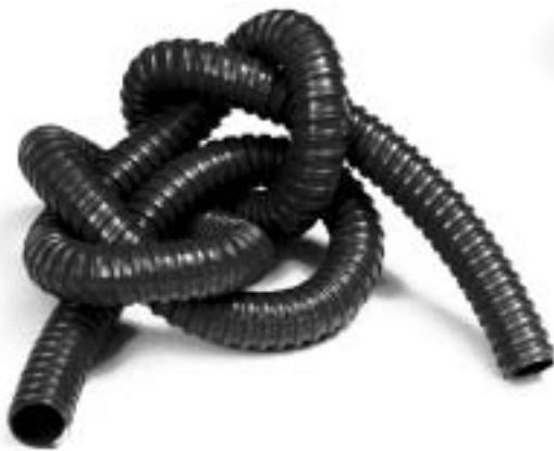
**Carflex X-Flex** Extra Flexible Nonmetallic Conduit is ideal for applications requiring extra strength and flexibility such as robotics, and repetitive flexing arms. Carflex X-Flex is nonconductive, noncorrosive, and resistant to oil, acid, ozone, and alkaline. It's designed for use with standard Carflex fittings providing a complete nonmetallic system. Carflex X-Flex is lightweight for easier handling, transportation, and installation.
