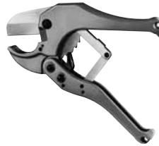
Hand held cutter makes fast square, smooth field cuts on conduit from 1/2" through 1 1/4". Produces burr-free cut with no shavings. Fits into pocket or pouch.
