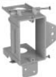
Open-backed to easily accommodate the bend radii required for low voltage cabling and deep devices such as volume controls, and is designed to fit a standard one-gang faceplate. It also features an easy nail-on mounting or screw-in bracket, while the hard shell provides increased durability and no racking. Resi-Rings accept 3/4", 1", and 1 1/4" Resi-Gard.
