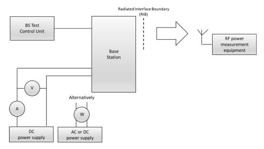
NOTE: BS as defined in Figure 2 (distributed BS). AC supply to be used for BS with build in AC power supply, otherwise default DC supply voltage as specified in clause 5.2.
