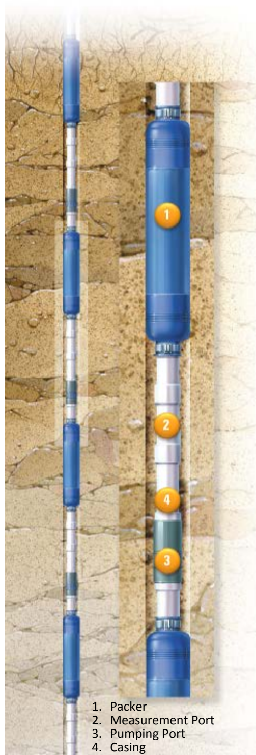
Figure 2.9 Typical Westbay Monitoring Well
