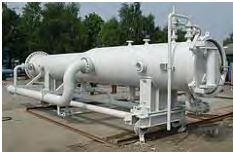
Figure 7: Typical PIG Launcher / Receiver Facility
