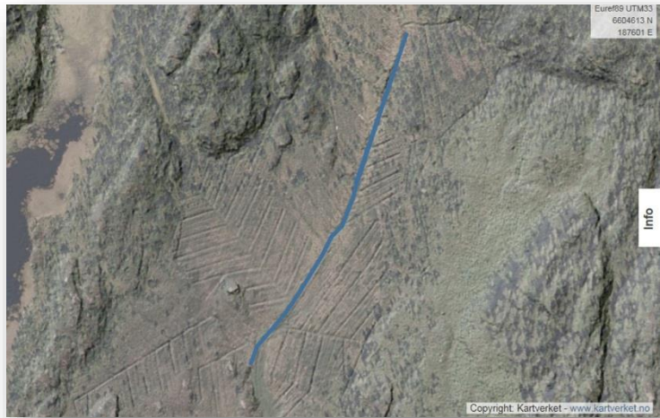
Figure 5 Aerial photograph of the upper mire detailing the modified stream and showing extensive herringbone ditches
