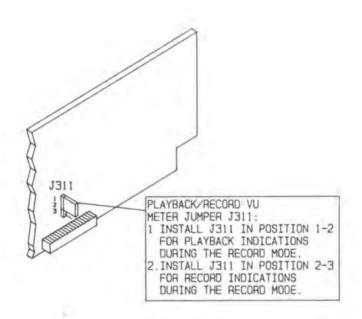
COPYRIGHT © 1990 BROADCAST ELECTRONICS, INC 597-9100-161 FIGURE 2-2. RECORD CIRCUIT BOARD JUMPER PROGRAMMING
