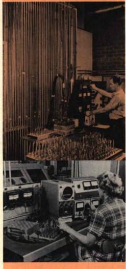
Electrical testing of silicon rectifiers, showing two of more than 27 in-process manufacturing tests.
