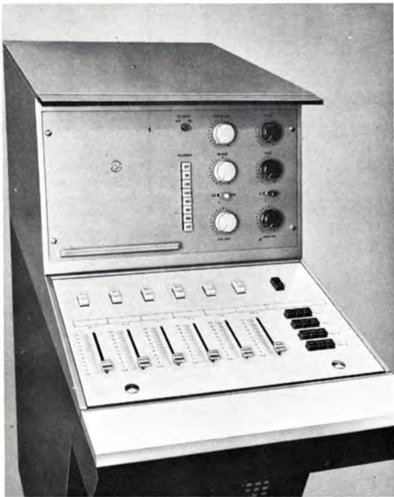
The record mixer and monitoring facilities offering control for two cartridge tape, two reel type tape machines and two turntables are contained in the third console. Solid state DC circuits and voice operated relays are highlighted in the equipment.
