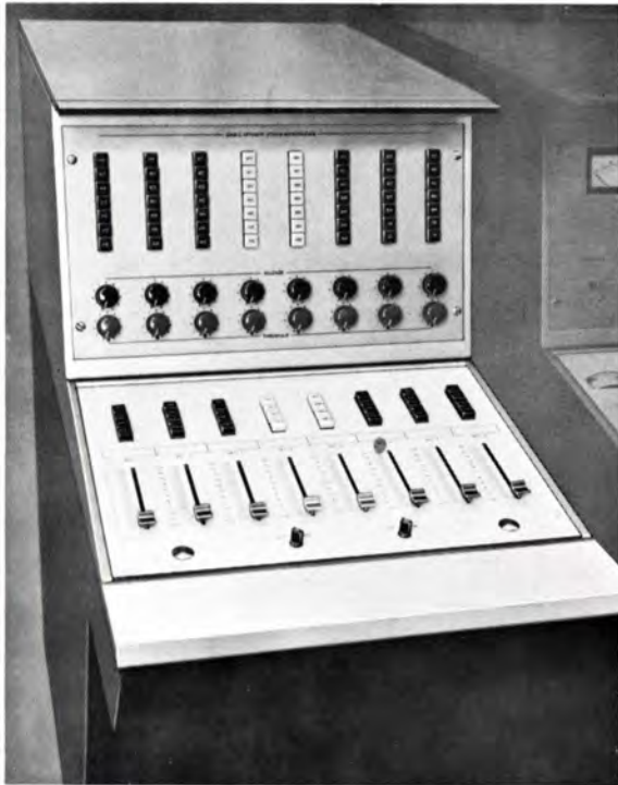
Three console housings designed for in-line installation will offer Station KRON complete studio audio facilities. Shown at left is eight-channel microphone mixer with three sub-mixing channels. Up to six microphones per channel can be selected. Note the vertical type faders, convenient bus selectors, and reverberation and equalizer controls. The second section is an eight-channel master mixer featuring latest RCA remote AGC meters and BA-40 series amplifiers.
