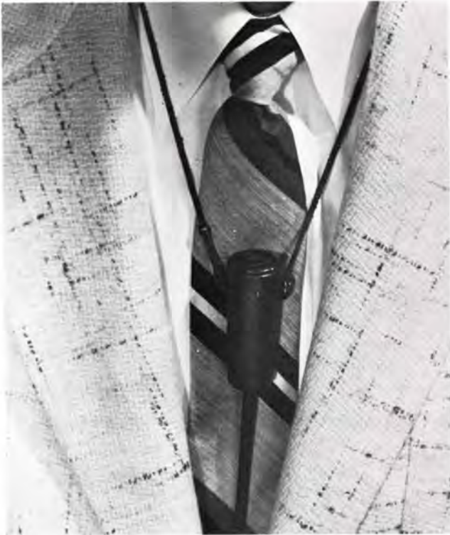
BK-6B Microphone used as a "necktie" mike. May be positioned beneath the necktie or exposed.
