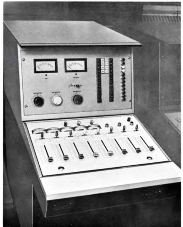
Three console housings designed for in-line installation will offer Station KRON complete studio audio facilities. Shown at left is eight-channel microphone mixer with three sub-mixing channels. Up to six microphones per channel can be selected. Note the vertical type faders, convenient bus selectors, and reverberation and equalizer controls. The second section is an eight-channel master mixer featuring latest RCA remote AGC meters and BA-40 series amplifiers.
