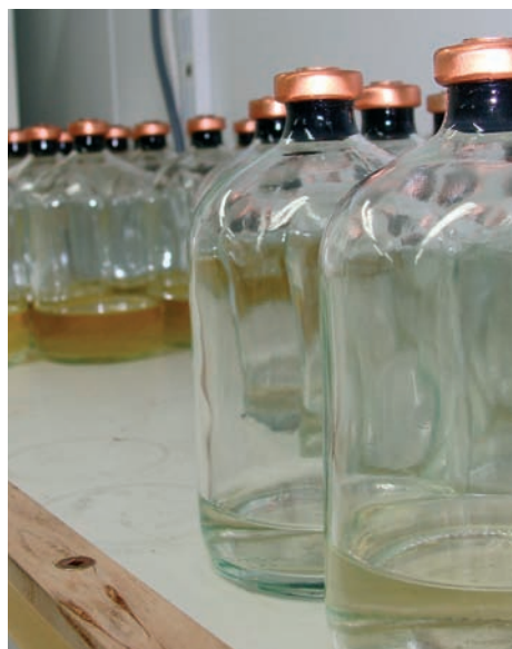
The microbes developed for the fermentation of CO to ethanol in converter waste gas are tolerant to variable concentrations of CO and the presence of N 2 and H 2
