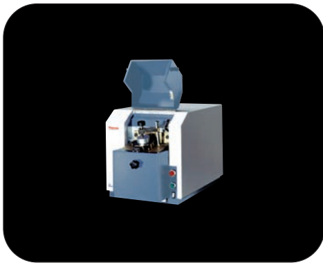
OES: Thermo Scientific ARL QuantoDesk CCD benchtop spectrometer
