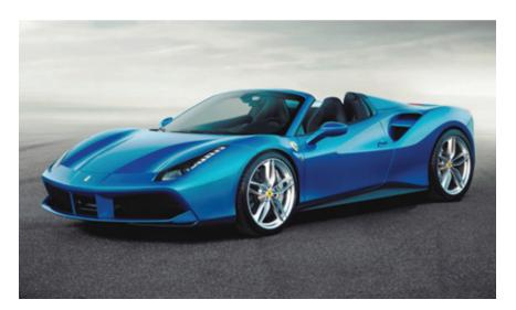
Our latest sports car, the 488 Spider, launched in September 2015, is a two seat coupe with a 670 hp mid-rear mounted V8 engine and is replacing the 458 Spider. Its retractable hard top, which saves approximately 25 kg on a soft top, unfolds and retracts in 14 seconds and can also be raised or lowered while the car is moving. Designed around the retractable hard top concept, the 488 Spider combines the prowess of the 488 GTB coupe's
