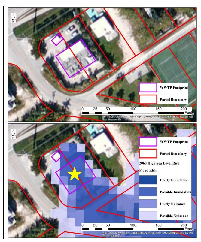
**Figure 10**: **Duck Key Wastewater Treatment Plant**. Aerial photograph (top) and 2060 high sea level rise assessment (bottom). Yellow star indicates structure with flood risk.
