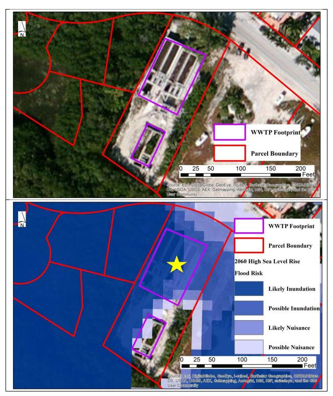
**Figure 9**: **Bay Point Wastewater Treatment Plant.** Aerial photograph (top) and 2060 high sea level rise assessment (bottom). Yellow star indicates structure with flood risk.
