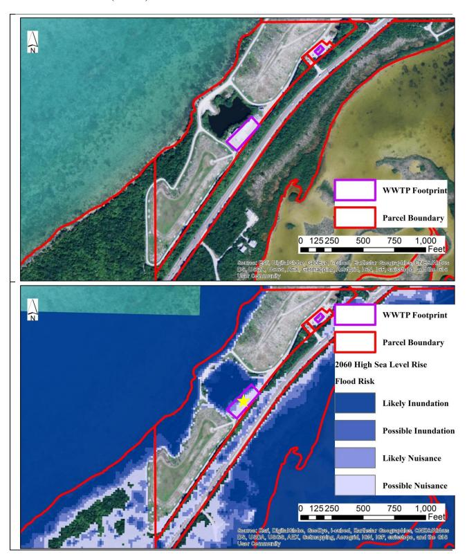
**Figure 13: North Key Largo Wastewater Treatment Plant**. Aerial photograph (top) and 2060 high sea level rise assessment (bottom). Yellow star indicates structure with flood risk.
