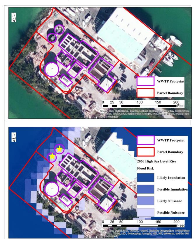
**Figure 11**: **Cudjoe Regional Wastewater Treatment Plant.** Aerial photograph (top) and 2060 high sea level rise assessment (bottom). Yellow star indicates structure with flood risk.
