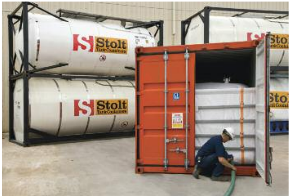
Inside a steel bulkhead, a flexitank is filled to the correct level.
