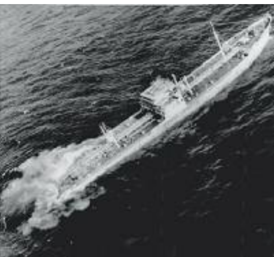
Protected by a bulkhead forward of the point of collision and the buoyancy of its cargo, Stolt Dagali ’s bow section remained afloat and was subsequently towed into New York Harbor.
