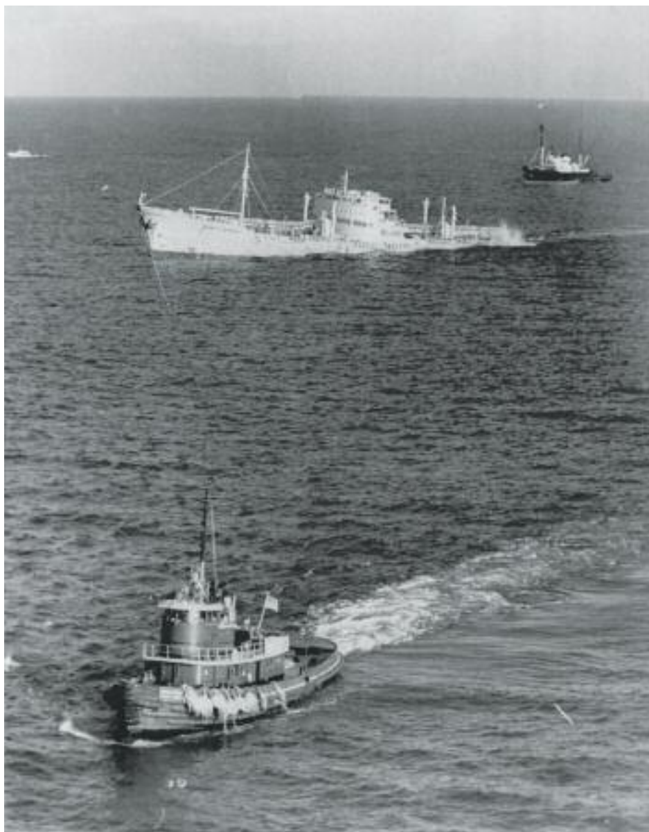
Protected by a bulkhead forward of the point of collision and the buoyancy of its cargo, Stolt Dagali ’s bow section remained afloat and was subsequently towed into New York Harbor.
