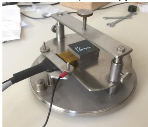
Figure 5. Measuring sensor sandwiched between two halves of a sample during measurement.
