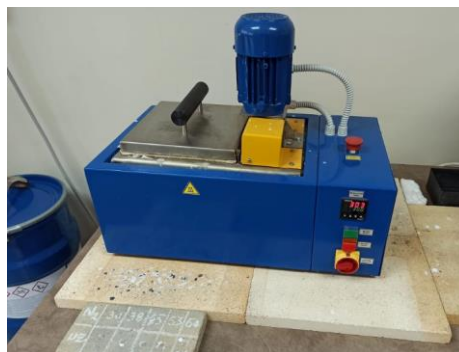
Figure 6: Salt bath furnace JPA 6-600
