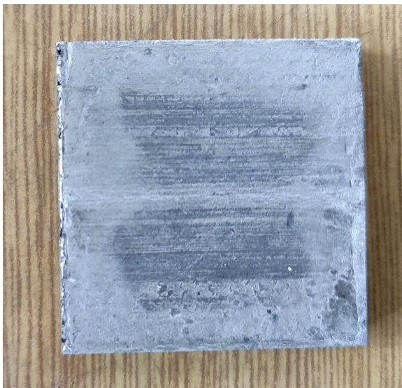
Figure 1: Aluminium foam with the dimension 40 \times 40 \times 5 \text{ mm}^3
