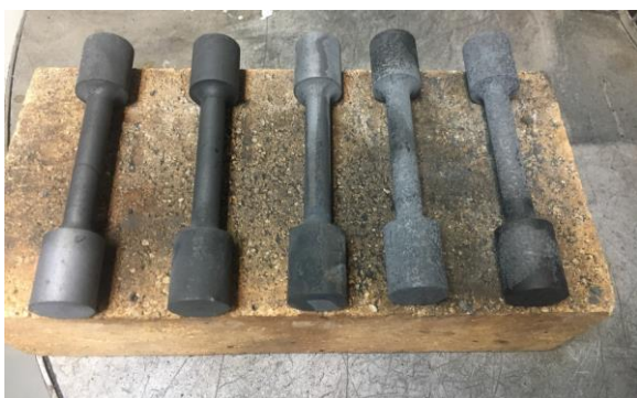
Figure 5: ADI samples after high temperature tempering
