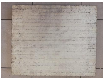
Figure 7. Aluminium foam panel with the dimensions 480 \times 400 \times 10 \text{ mm}^3 and weight 2138 g made of a foamable precursor prepared from fine-grained aluminum powder of 99.7% purity with a grain size of less than 63 \mu\text{m} with a content of 0.15 wt. % of \text{TiH}_2 powder as a foaming agent (panel density: 1.11 \text{ g/cm}^3 ).
