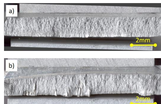
Figure 1. Longitudinal fractures of the 1.8 mm thick AA5056 alloy joints obtained by FSW (a) and GTAW (b)
