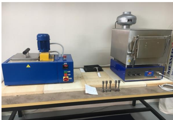
Figure 4. Austempering salt bath (left) and austenitization furnace (right)
