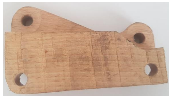
Figure 3. Initial wooden model of the bracket
