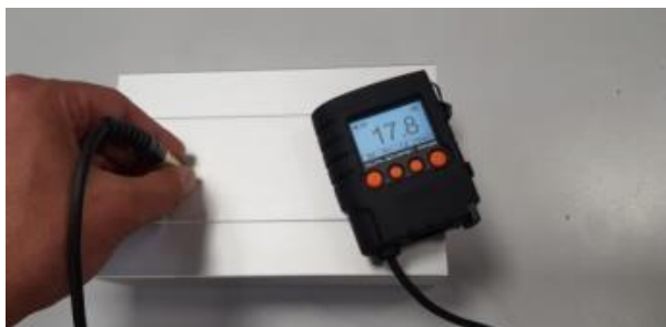
Figure 16. Eddy current height/width measuring gauge [21]
