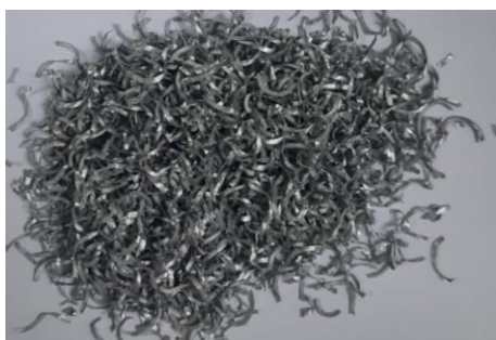
Figure 1. Aluminium alloy A380 chip waste
