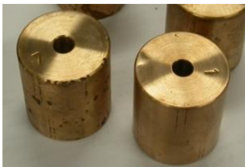
Figure 3. Disks from ground and molded rapidly solidified Cu-Al-Ni-Mn shape memory alloy.
