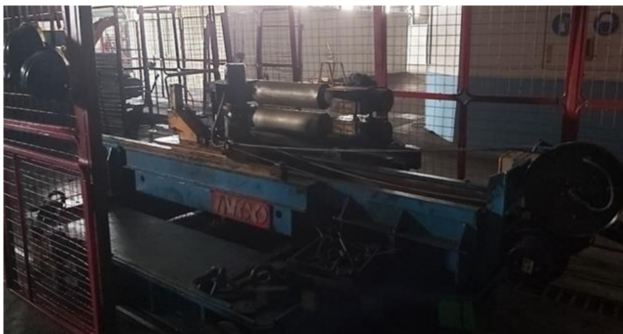
Figure 2. Device for mechanized replacement of working roller
