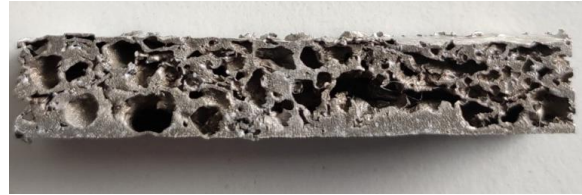
Figure 2: Pores formation inside aluminium foam (cross-section)
