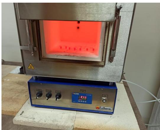
Figure 4: Austenitization of test samples on 850^\circ\text{C}
