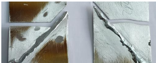
Figure 3. Aluminium strip soldered joints break at HAZ: a) scarf joint (unbrushed covered with paint) a) scarf joint (brushed and acetone cleaned)
