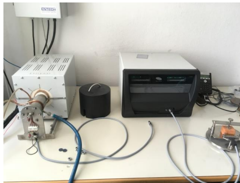
Figure 4. Instrument Hot Disk TPS 2200.
