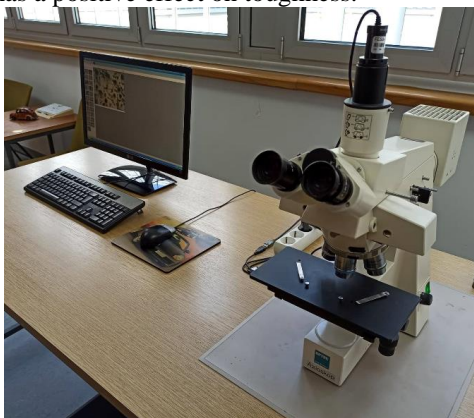
Figure 8: OPTON Axioskop light microscope
