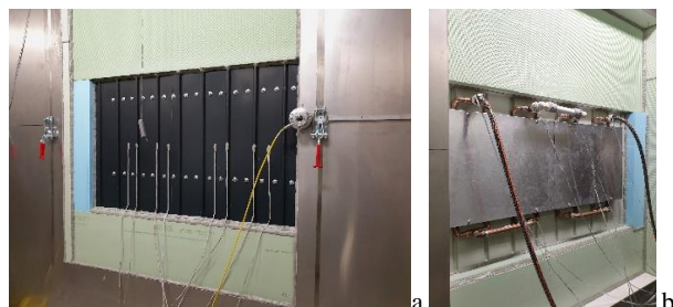
Figure 8. View of tested roofing tiles in a climate chamber for modeling of synergic effects of heat transfer, water vapor diffusion, and air filtration from the exterior (a) and interior side (b).
