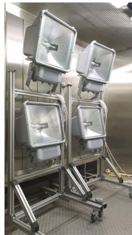
Figure 9. The solar system consisting of four reflectors of the Lightmaster 1000 CL1 type fitted with Osram HQI-TS 1000 W / D / S PRO lamps.
