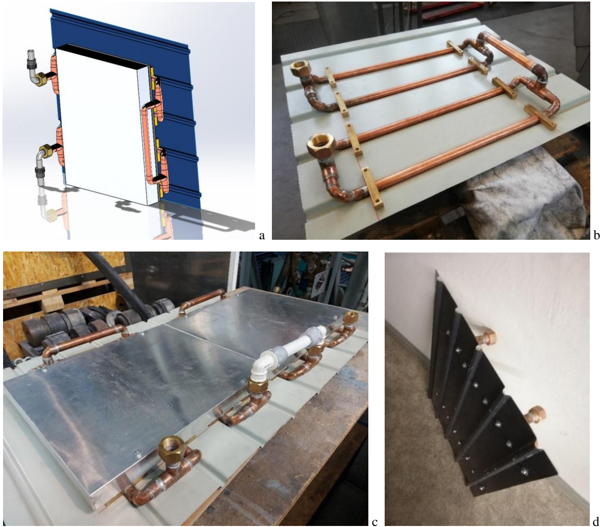
Figure 5. Prototype of a functional demonstration area with dimensions 680 \times 1060 \text{ mm}^2 covered with two pieces of roofing tiles (a) bottom view of a virtual model of roofing tile; (b) view of the piping system of heat transfer fluid distribution with copper pipes; (c) view of interconnected 2 prototype roofing tiles from below; (d) view of the part of the prototype roofing with the integrated function of the heat exchanger from the side of the covering surface trapezoidal sheet.
