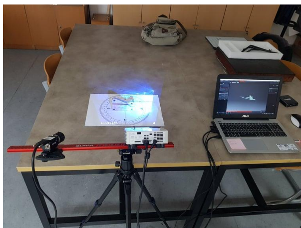
Figure 4. 3D scanning of the brake caliper bracket
