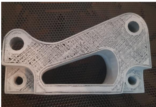
Figure 17. Results of second 3D printing from both sides
