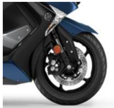
Figure 1. Factory brake disc 267 mm, [8]
