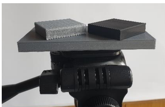
Figure 2. Experimental setup for measuring the slip angle
