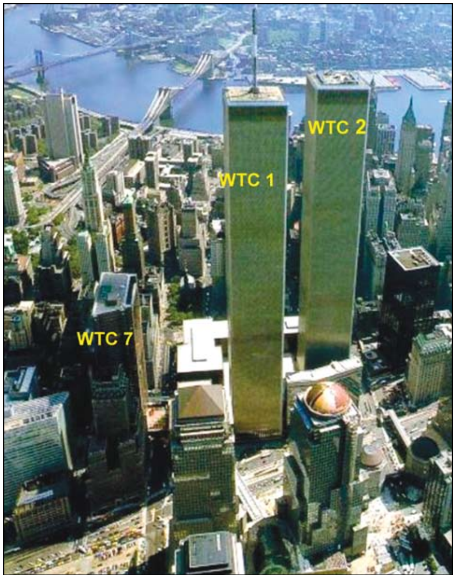
World Trade Center 7, on the north side of the World Trade Center Complex. The collapse of WTC 1 sent flaming debris into the southern face of WTC 7 and initiated a chain of events that would eventually lead to collapse.
