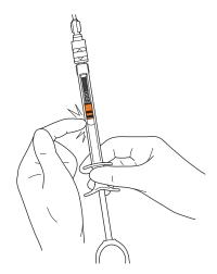
1.8. While still pointing the syringe tip towards the ceiling, push the plunger all the way in (Figure 2), to purge all air and fluid from the syringe.
