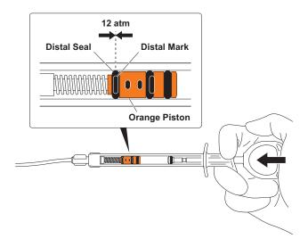
Figure 5 – Alignment between Distal Seal and Distal Mark corresponds to 12 atm
