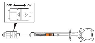
Figure 1 - Inflation lock attachment and positions
