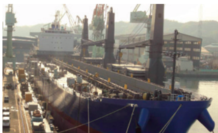
Specialized vessel for transporting long rails (150 meters in length)
