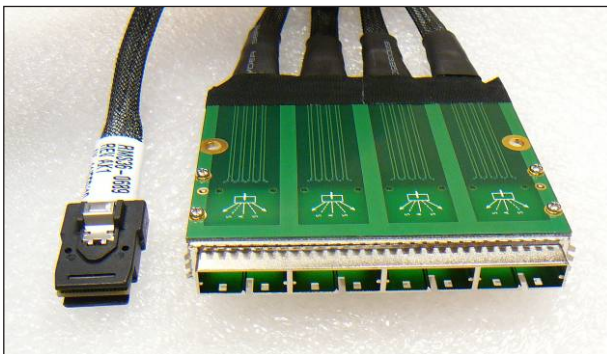
Figure E-5: Up-Close of the Special Connector Cable Board
