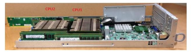
3. Remove the original bracket from the node.
