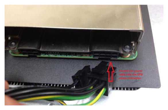
10. If your GPU has two power connectors, please insert the second power cable as shown below.
