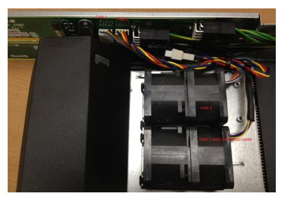
5. Connect FAN1 and FAN2 to the FAN1 and FAN2 connectors on the power adaptor card.
