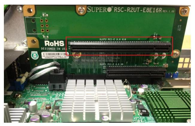
6. Insert the gold contacts on the GPU intoPCIe slot2 on the riser card.
