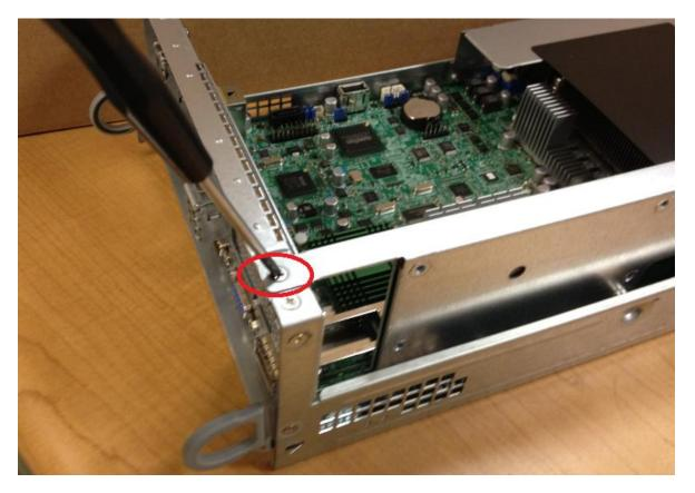
• Confirm four screws are secured on the bracket.
