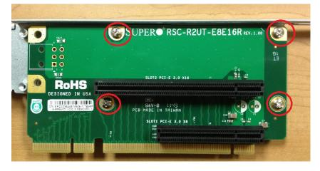
3. Confirm that six screws are now attached to the support bracket.
