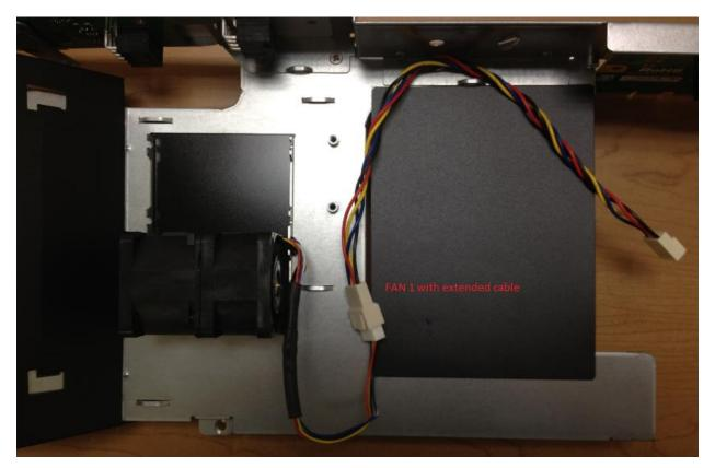
4. Locate FAN1 and FAN2 connectors on the power adaptor card (above, Rev. 1.02)
