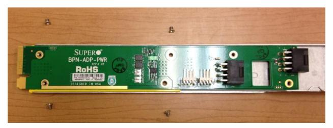
8. Secure the power adaptor card and plate to the bracket with the four screws shown as below.
