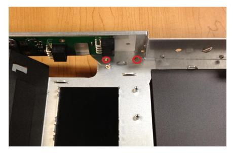
3. A thin phillips screwdriver is necessary to secure the screw in this position.
