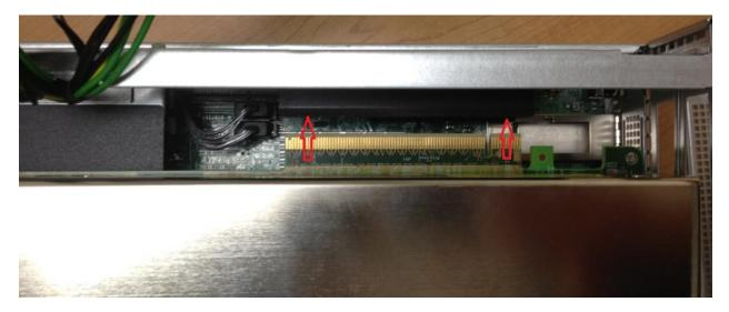
7. Slide the sheet metal piece from left to right after the GPU is installed.
