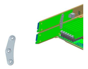
1. Follow the procedure below to attach the power adaptor card to the SATA backplane using three (6mm screws).
