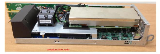
Completed the GPU kit with GPU correctly installed.
