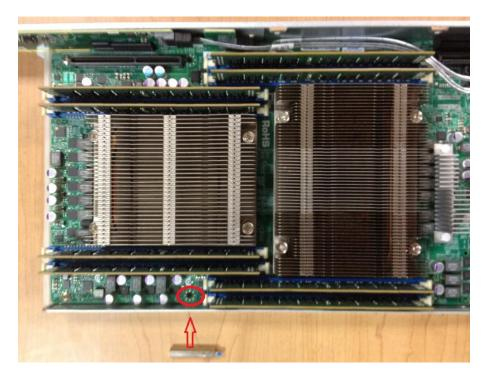
5. Insert the riser card into the PCIe x 16 slot on the motherboard.
