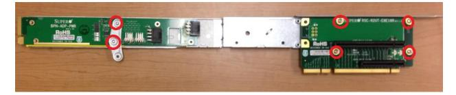
Attaching the Motherboard tray support bracket to the power adaptor & riser card support bracket:
