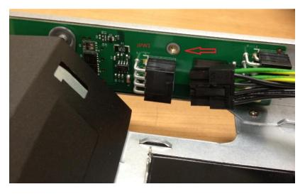
3. Insert the 2+6 pin connector into JPW2.
