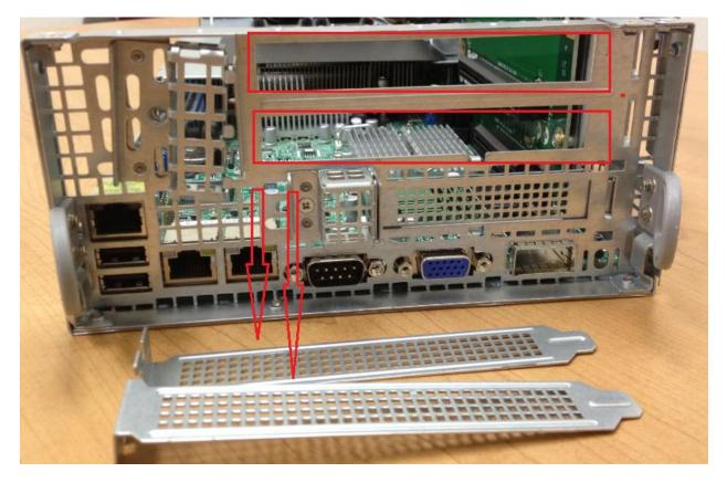
2. Loosen the screw and slide the piece from right to left.
