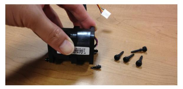
2. Insert the fan into the motherboard tray support bracket.
