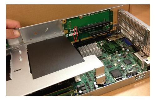
6. Secure the motherboard tray support bracket with two 3mm screws.
