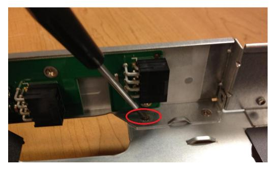
4. Secure the MB tray assembly and power adaptor card & riser card bracket firmly secured together.
