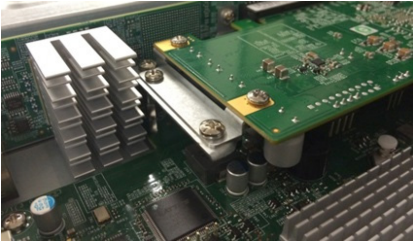
Figure 6-10. Installing the Internal Expansion Card
