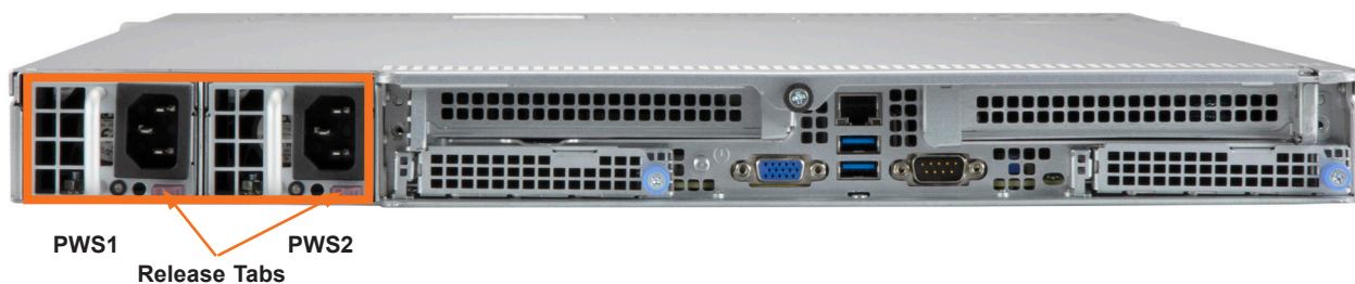
Figure 3-12. Replacing the Power Supply
